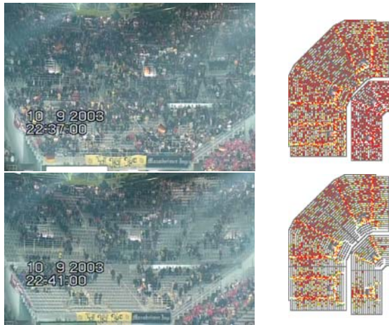
Fig. 4. The Westfalenstadion Dortmund: Comparison of the results for the video analysis (left column) and the simulation (right column) at the beginning of the egress. The video snapshots are taken at (from top to bottom) t = 2 and t = 6 minutes for the videos and t = 20 seconds and t = 3 minutes for the simulation.
