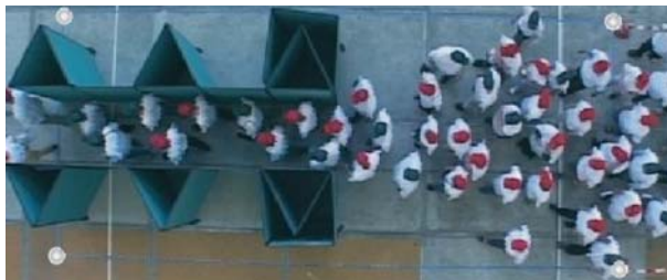
Fig. 1. Overview of the narrow bottleneck experiment.
