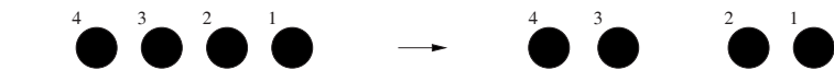
Fig. 1. Shuffled update of a cluster consisting of four particles numbered from right to left. The drawn sequence is 3, 4, 1, 2 and p = 1 .
