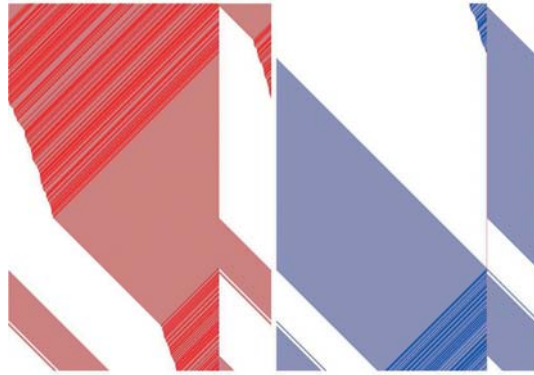
Fig. 4. A spatiotemporal pattern of cars advancing on the X-road (left) and Y-road (right), respectively. Cars move to the right and time increases from top to bottom. The number of cells is L = 500 and the intersection is located at L = 100 from the right edge.
