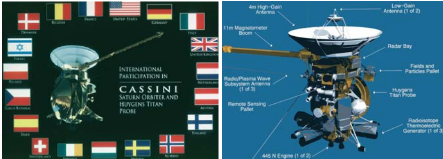
Fig. 5. The Cassini mission. The Cassini Huygens mission is an international collaboration. The flags of the participating countries are represented on the left. The Cassini orbiter (right image) carries 12 instruments. The overall height of the assembled spacecraft is 6.8 metres and its weight is 5.7 tons. (NASA-JPL/ESA documents).
