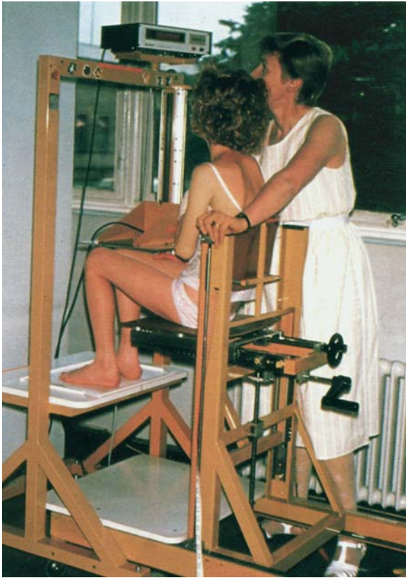
Fig. 11.46. A knemometer. The child is positioned so that the knee is positioned at a right angle and the feet are comfortably placed. At the first visit a template is made by drawing around the child's feet, so that at the subsequent visit positioning is identical.
