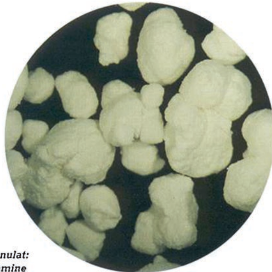
Fig. 9.4 Typical example of a high shear granulate (courtesy of Glatt GmbH, Binzen, Germany, www.glatt.de )
