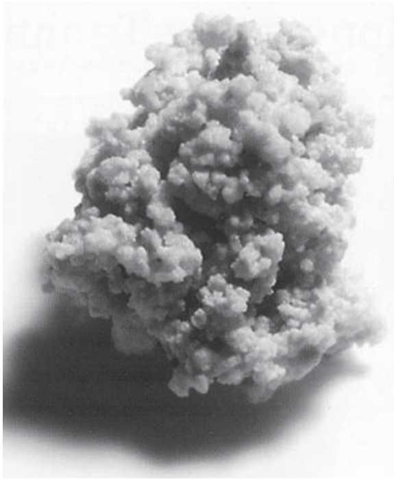
Fig. 9.11 Typical example of fluid bed agglomerate (courtesy of Glatt GmbH, Binzen, Germany, www.glatt.de )
