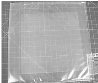
Figure 11-9 Nafion 115 membrane (courtesy of Fuel Cell Scientific [38]).
