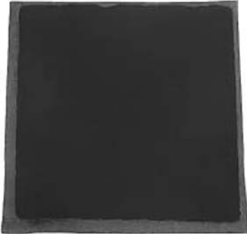
Figure 11-10 A PEMFC electrode (courtesy of Fuel Cell Scientific [38]).
