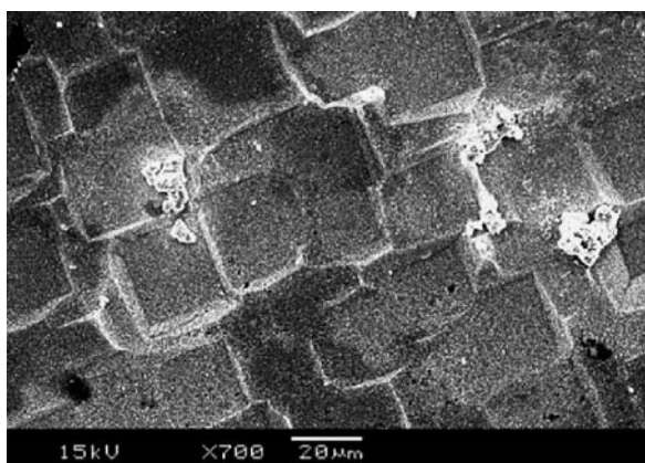
Fig. 4.3 SEM micrograph of the rear side of an n-(100) Si wafer polished on one side. The presence of inverted truncated square pyramidal structures fully covering the surface can be observed. This pyramidal texturing was attributed to the combination of anisotropic etching of the silicon and to hydrogen bubbles evolved during the etching reaction. (Reprinted from [23] Copyright 2009, with permission from Elsevier)
