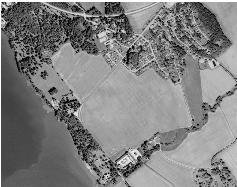
Fig. 14.1 An aerial photograph with 4 m resolution over Julita, in mideastern Sweden ( \sim 2 \times 2.5 km). The photo is an orthophoto, meaning that it has been geometrically corrected. Agriculture, deciduous forest and shelterbelt trees can be detected as well as individual houses and gardens. The area in the lower left corner is part of Lake Öljaren. (Courtesy of Lantmäteriet Gävle 2007. Medgivande I 2007/437)
