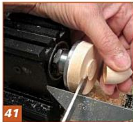
41 Create a tenon on a waste block to fit the interior.
