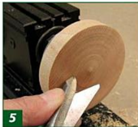
5 Adjust the tool rest to provide support for the tool as the cut is made across the face.
