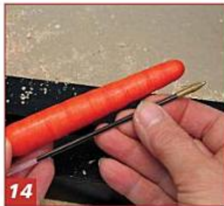
14 Measure the drilled hole for depth, shorten the insert with scissors if needed, and push the insert into place.
