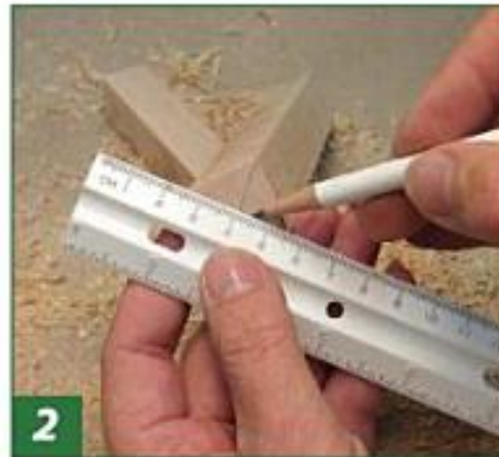
2 Locate the center of the blank for the live center point, using a ruler held across the corners.
