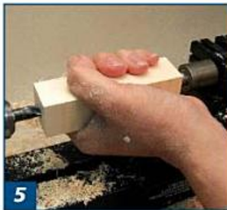
5 Holding the workpiece securely, use the tailstock to push it onto the drill bit with the lathe running. Clear the chips as necessary to allow efficient cutting.
