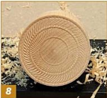
8 This is some chatterwork done at about 2,000 rpm. You typically get a finer pattern with a slower speed.
