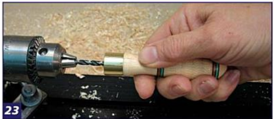
23 Drill the hole for the tool by holding the handle parallel to the lathe bed and pushing it onto a spinning drill bit driven by the headstock, or use a drill press. If you know ahead of time what tool you are making the handle for, you could predrill the correct size hole instead of the 1/8" pilot hole.
