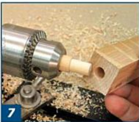
7 The tenon should fit the \frac{1}{8} " hole very tightly, as this will drive the workpiece. If you find that it slips, try moistening the tenon.
