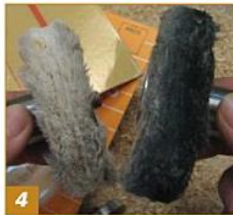
4 It is good to have a wheel dedicated for each different buffing compound used and a separate one just for items finished with black India ink.
