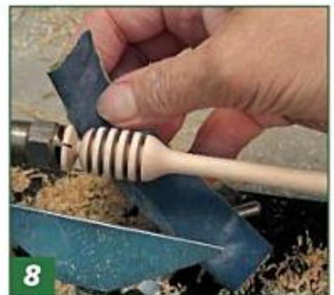
8 Sand the end of the dipper after reducing it to the desired diameter.
