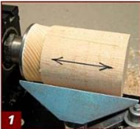
1 Mount the workpiece on a glue block with the grain parallel to the lathe.
