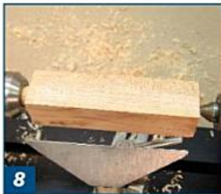
8 Mount the workpiece between centers, seated all the way onto the tenon, and turn it round using the \frac{1}{8} " gouge.
