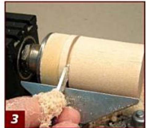
3 About \frac{1}{8} " to the right of the glue line, make a parting tool cut.
