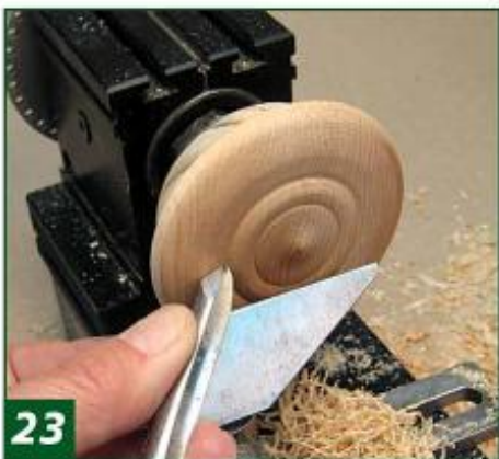
23 Shape the back, with the tool rest oriented across the workpiece for tool support.
