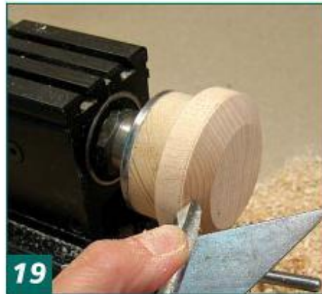
19 Start shaping each half. Use the line to help shape each half identically.
