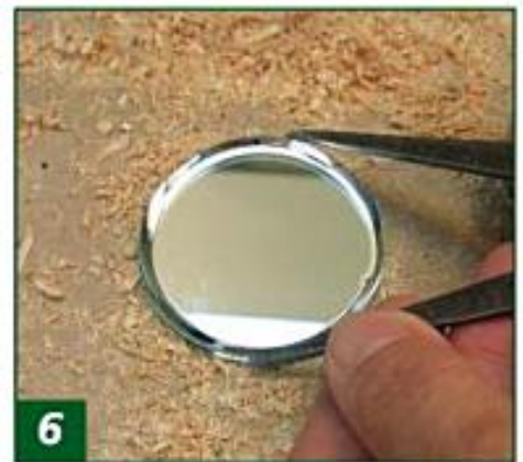
6 Set a pair of dividers to the diameter of the mirror.
