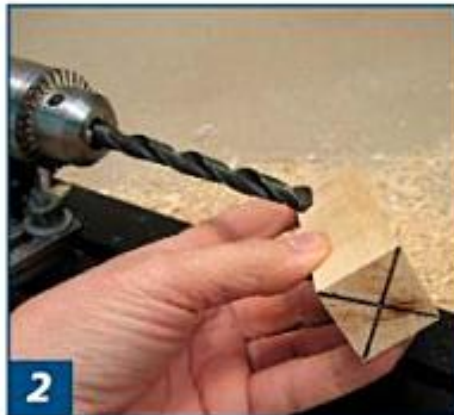
2 If you would like to drill the hole on the lathe, locate the center for the tailstock end.
