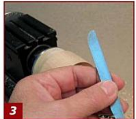
3 The round nose scraper has been sharpened on the end and along the side.
