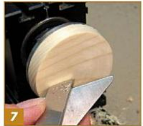
7 Until you gain the expertise with the gouge to make the surface flat enough for a glue joint, you could do some leveling with the skew chisel lying flat on the tool rest. Keep practicing with the gouge.
