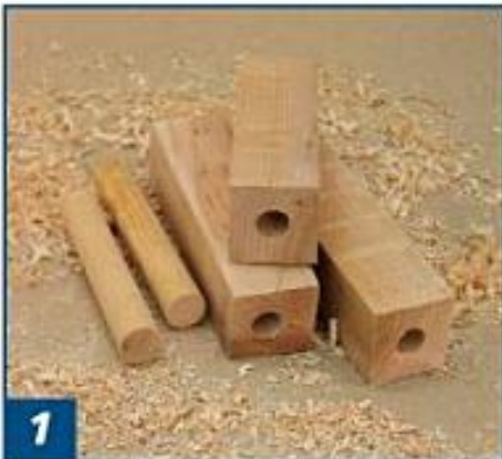
1 Predrilled whistle blanks and \frac{1}{8} " dowels.
