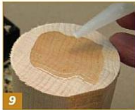
9 Use a medium or thick CA (cyanoacrylate) glue on one piece of wood and spray the accelerator on the other piece.
