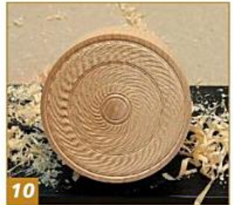
10 The tip of a skew lying on its side has been used to accentuate the pattern in Photo 9 with some small grooves.
