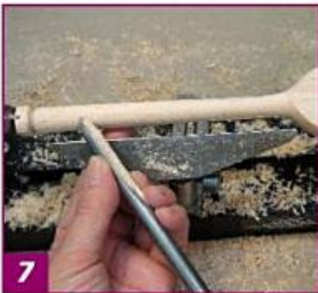
7 You could speed up the lathe a bit as you turn the handle down to the desired diameter.
