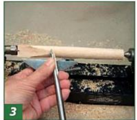
3 Mount between centers and turn the workpiece down to round using a \frac{1}{8} " gouge.
