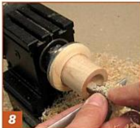
8 Continue hollowing to a finished depth of about \frac{1}{8} ".
