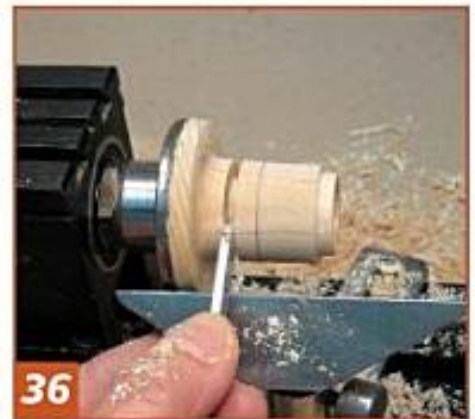
36 Make a parting tool cut, allowing extra wood for shaping the nut.
