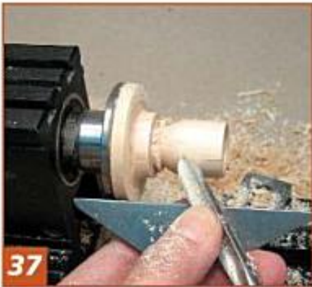
37 Use the gouge to cut the sides down to the diameter of the tenon.
