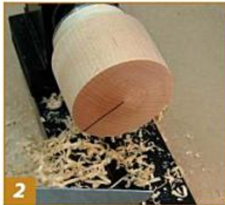
2 On the end of a practice piece of dense wood (with the grain parallel to the lathe), draw a line from the center to the edge. Rotate the line to where a clock hand would be at 7:30.
