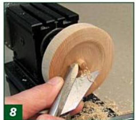
8 Start removing wood with the gouge (bevel rubbing), leaving a small stump in the center to serve as a temporary depth gauge. The recess needs to be about \frac{1}{8} " deep.
