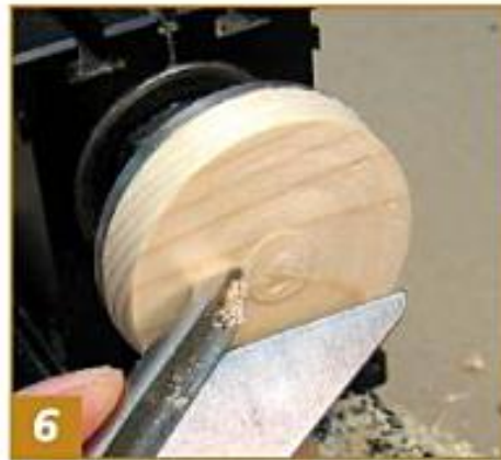
6 Flatten the face after adjusting your tool rest to support the tool for the entire cut.
