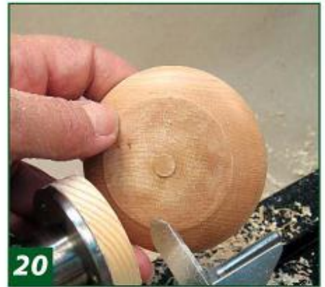
20 If you part right at the glue line, there won't be much clean-up needed.
