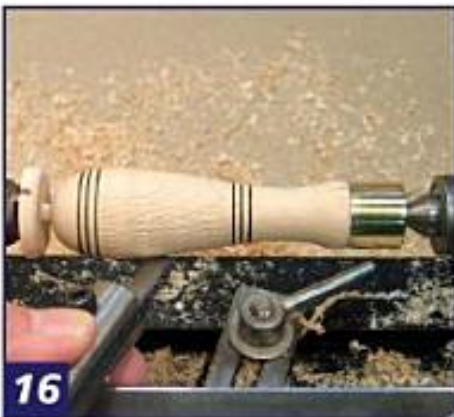
16 Add some interesting texture with the chatter tool. (See the side chatter tips on pages 7–8.)
