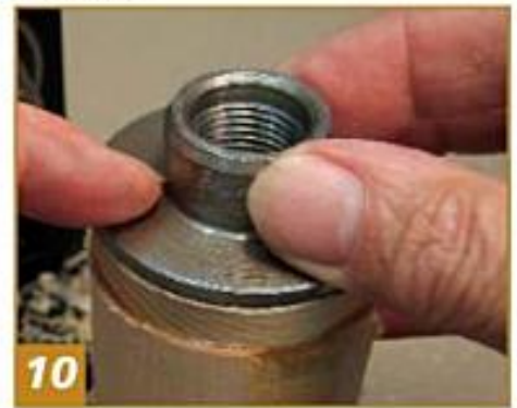
10 Put the two together and hold for a few seconds until the glue sets. Before turning the lathe on, spray some accelerator on any glue that squeezed out.
