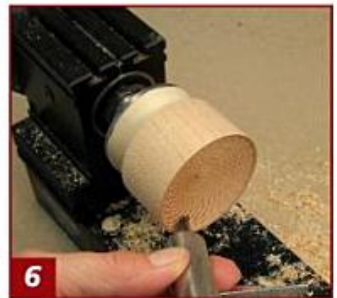
6 Use the chatter tool to create a pattern across the surface. To prevent the grain from splitting out, stop before you get to the edge.
