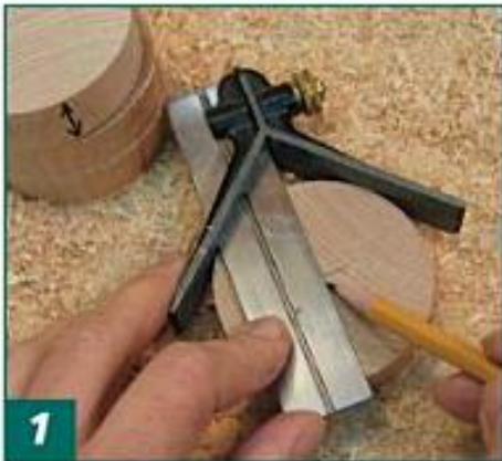
1 To prepare the end-grain blanks, locate the center of each half. Arrows show grain direction.
