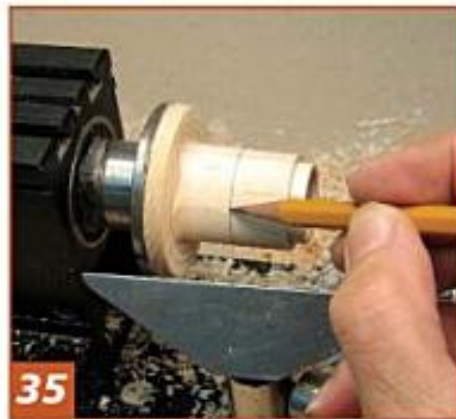
35 Mark the depth of the interior.
