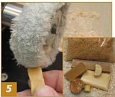
5 Carnauba wax is applied lightly to a spinning buff. Excess wax will cause white streaks in your finish. These can be removed by using a clean buffing wheel. Inset: Pure carnauba wax comes in many forms. Smaller pieces can be remelted and poured into a small mold.
