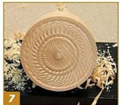
7 If you interrupt the movement of the tool, lift it off, move it over, and set it back down, you can create an un-chattered band for accent.
