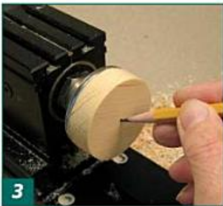
3 To prepare the mounting block or jig, face it off flat, locate the center, and create a small recess for the drill bit to center on.
