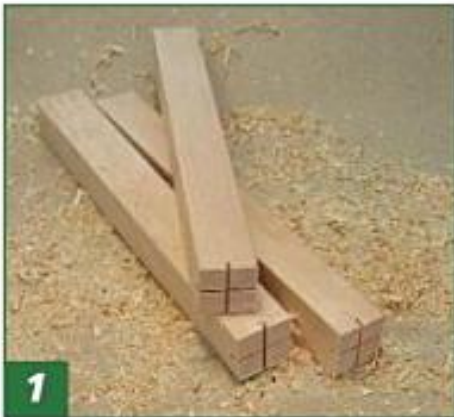
1 Three blanks prepared with bandsaw cuts for the spur drive.
