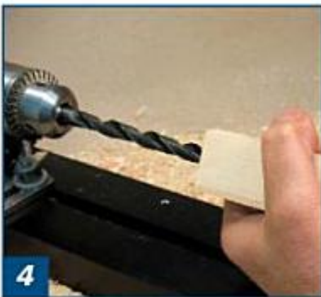
4 Hold the workpiece against the tailstock and aligned with the drill bit.
