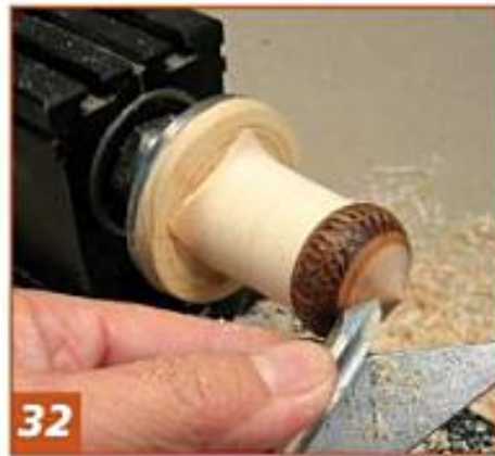
32 Press the cap on and do the final shaping for the tip.
