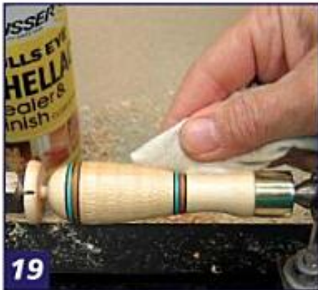
19 Seal the surface with spray shellac. Be careful not to smear the colors.
