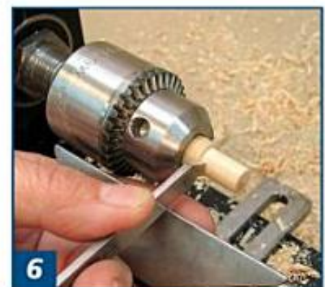
6 To make a plug for driving the workpiece, use a Jacobs chuck to hold a section of \frac{1}{8} " dowel with about 1" protruding. Turn a tenon about \frac{1}{8} " long with a square shoulder as a stop.
