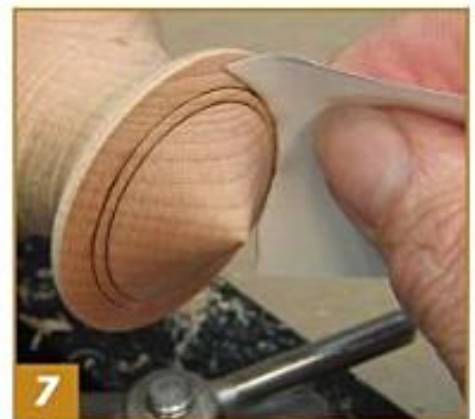
7 Use a piece of paper—20 lb or 24 lb—held in the groove until it burns. You will need to speed up the lathe and will know it is working when you see smoke. Heavier paper will be better for burning lines in larger grooves.
