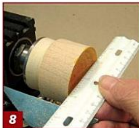
8 Use a straightedge to visually check the depth.
