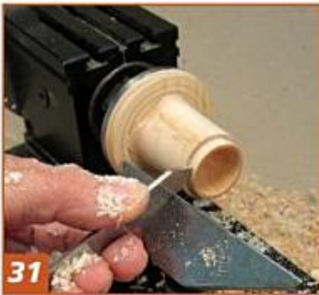
31 Lengthen the tenon to about \frac{1}{8} ", maintaining a tight fit.
