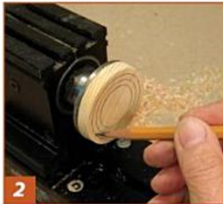
2 With the lathe running, use a pencil to make some concentric circles as a target. The target is helpful for centering your workpiece.
