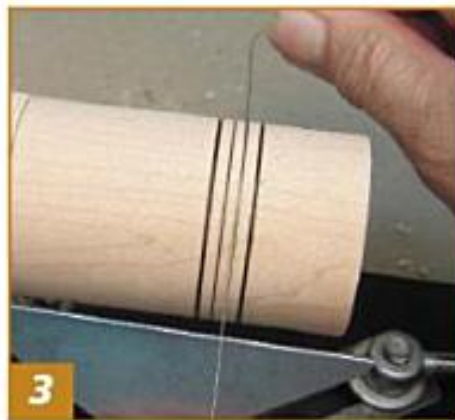
3 The two inner lines have been burned with a finer gauge wire—about 22g. Hold the wire against the piece without moving it back and forth.
