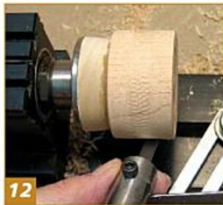
12 A chatter pattern can also be applied to the side of a workpiece by holding the tip of the tool low and under the workpiece.
