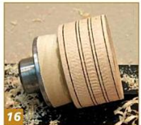
16 Make some grooves and burn some lines to enhance the pattern.
