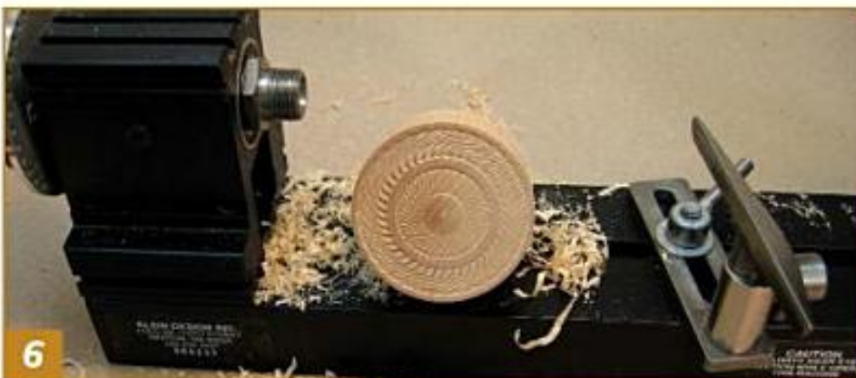
6 With a speed of about 2,000 rpm, touch the tip of the tool to the face of the workpiece about \frac{1}{8} " from the center. With light pressure, you should hear chatter. Too much pressure will just cut a groove. Move the tool (along the "7:30 line") adding pressure as the diameter increases. Pressure is increased as the surface speed increases.
