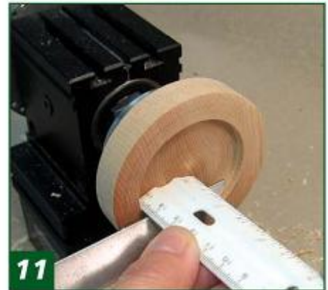
11 Check to see that the depth is \frac{1}{4} ", that the side of the recess is exactly parallel to the lathe bed, and that the bottom is flat.
