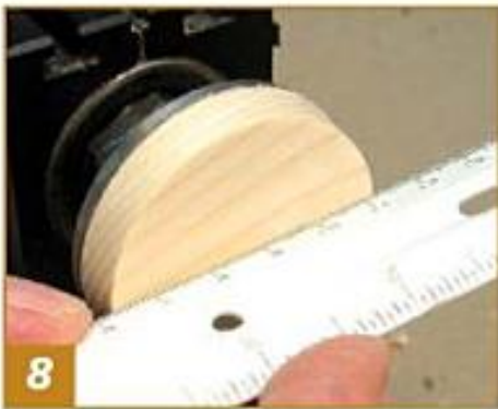
8 With the lathe off, check to see that your surface is flat.
