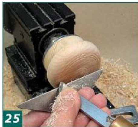
25 Use the tip of the skew to create small V-cuts to enhance the boundary lines.
