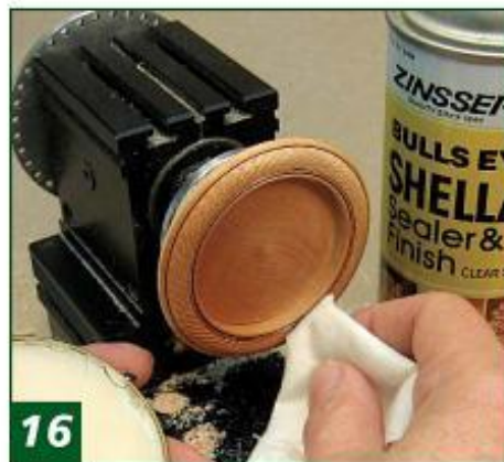
16 After sanding, apply some spray shellac as a sealer, making sure it penetrates the end grain chatterwork thoroughly, and then apply wax.
