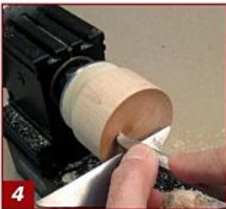
4 Create a shallow, concave recess about \frac{1}{8} " deep with the round nose scraper.
