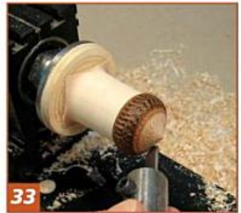
33 Use the chatter tool to apply texture.
