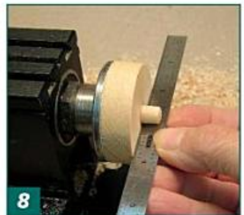
8 Check the face of the mounting block to be certain it is absolutely flat.
