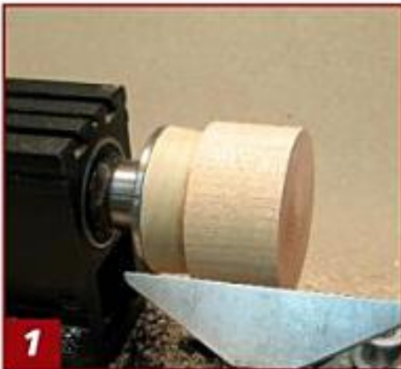
1 Preparation: Mount the block with the grain direction parallel to the lathe bed.
