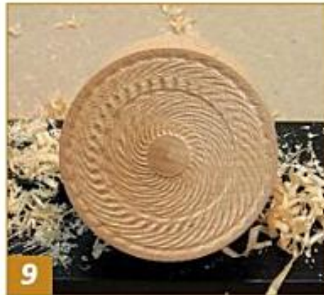
9 This is a pattern chattered at about 3,000 rpm.
