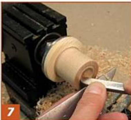
7 Start hollowing with the round nose scraper held flat on the rest.
