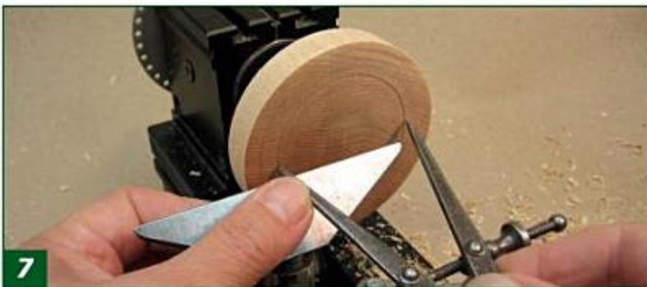
7 Transfer that measurement to the workpiece. With the lathe running and the left side resting on the tool rest, touch the wood with only the left point to create a line at the desired diameter when it appears under the right point of the dividers.
