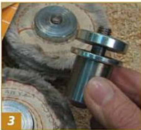
3 On the Klein Lathe, an arbor is used to mount the buffing wheel on the spindle. There are many types of arbors available for this use.
