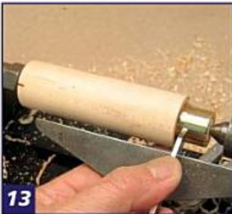
13 A parting tool will work also. The HSS tools will cut because they are much harder than the brass.
