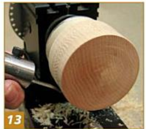
13 This is a side view. The chatter tool is pressed up against the workpiece.
