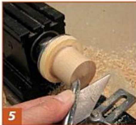
5 Adjust the tool rest to support the gouge for the cut across the face.
