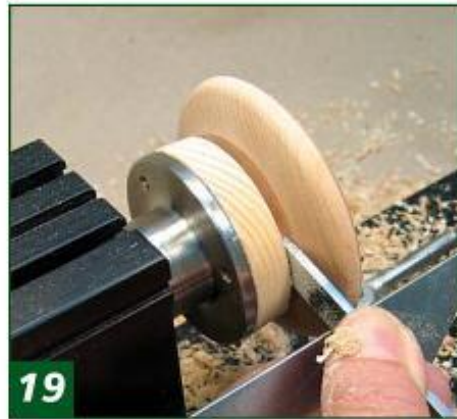
19 Part off the workpiece by cutting through the glue block.
