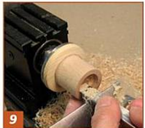
9 Using the left side of the square scraper, cut the inside parallel to the lathe bed, creating a step about \frac{1}{8} " deep.
