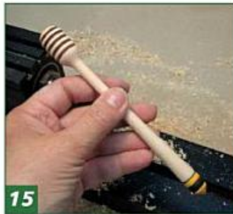
15 You can soak the dipper in mineral oil and wipe it dry as a finish, or you could buff it with carnauba wax on the buffing wheel.
