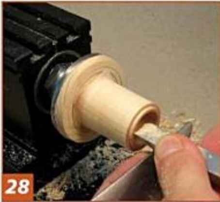
28 Straighten the first \frac{1}{8} " of the interior side walls with the square scraper. This will make it easier to do the reverse chucking for turning the tip of the nut.
