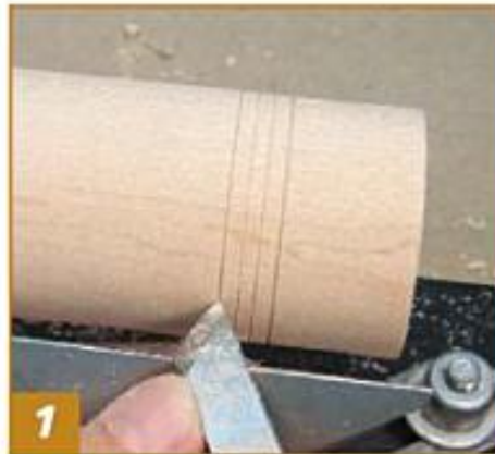
1 On a practice piece of wood, use the tip of a skew lying on its side to make a few grooves.
