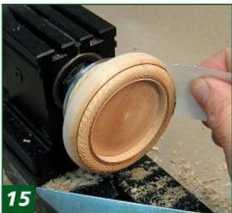
15 The edge of a small piece of paper held in the grooves with the lathe running at a fast speed will create nice, decorative burn marks. (For more information on this technique, see page 6)
