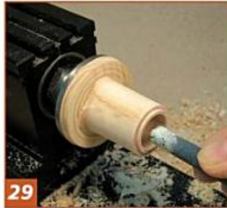
29 Sandpaper wrapped around a pencil works well for sanding the inside.
