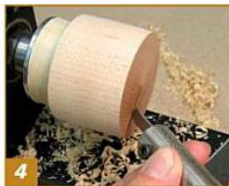
4 This is the front view. The tool shaft is supported by the tool rest, and nothing should be touching the blade.
