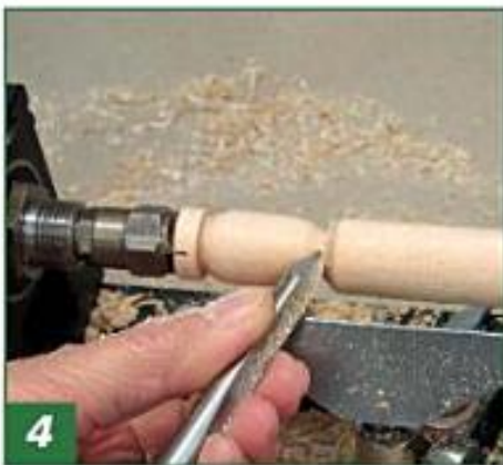
4 Use the \frac{1}{8} " gouge to shape the dipper part, but to maintain support, don't make the neck or the waste wood near the spur too narrow at this time.
