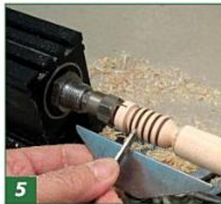
5 With a parting tool, cut several slots, evenly spaced, down to about \frac{1}{16} " in diameter. A thinner parting tool may make more attractive slots.
