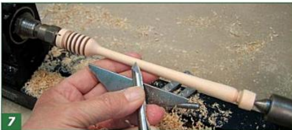
7 Finish shaping the handle before turning a couple of beads for the honey bee's body. Leave a little waste wood for sawing off. Use your finger for support to prevent wood movement.
