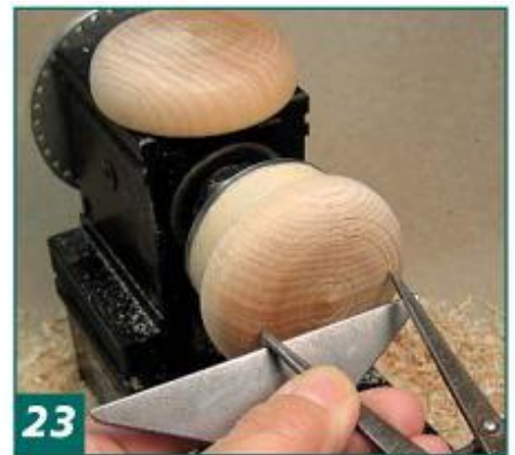
23 Use dividers to mark identical lines on each piece.
