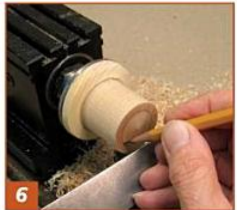
6 Mark off about \frac{1}{8} " diameter for the interior of the cap. The outside diameter is about 1\frac{1}{4} ".
