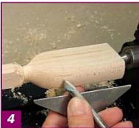
4 Using the \frac{1}{8} " gouge, start by shaping the spatula end. Turn that area down to the desired shape.
