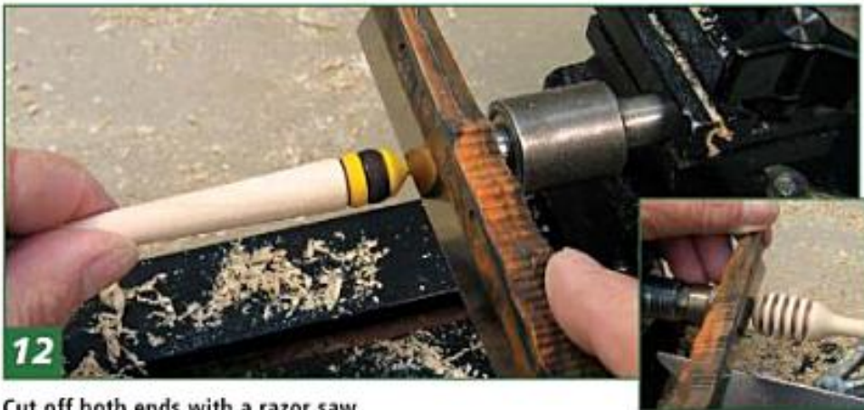
12 Cut off both ends with a razor saw. Do this with the lathe turned off.
