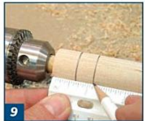
9 Mark off a section \frac{1}{8} " long for the mouthpiece and another section \frac{1}{8} " long for the notch area.
