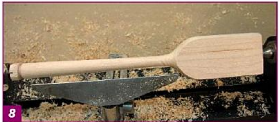
8 When you are turning long, thin spindles, you may get a spiral pattern. This is caused by wood movement as a result of excess tool pressure or possibly of worn or poor quality bearings in the live center. If you like the pattern, you could keep it. See the Spiral Chatter Eggs section on page 28 for more information.
