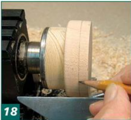
18 Draw a reference line on the circumference of each half an equal distance from the face.
