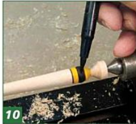
10 Apply the black color to the bee body. Burned lines help to prevent colors from running.
