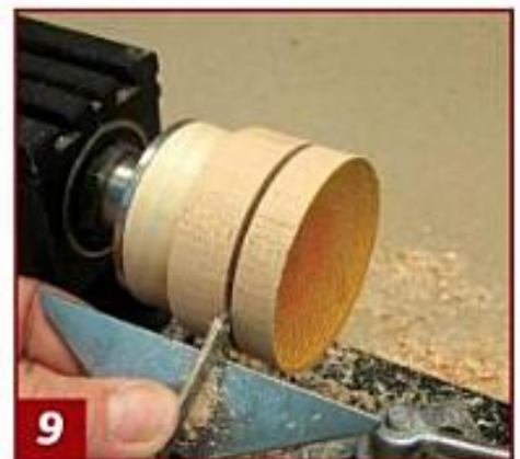
9 Make a parting tool cut down to about a \frac{1}{8} " diameter, adding about \frac{1}{16} " in depth for the thickness of the earrings.
