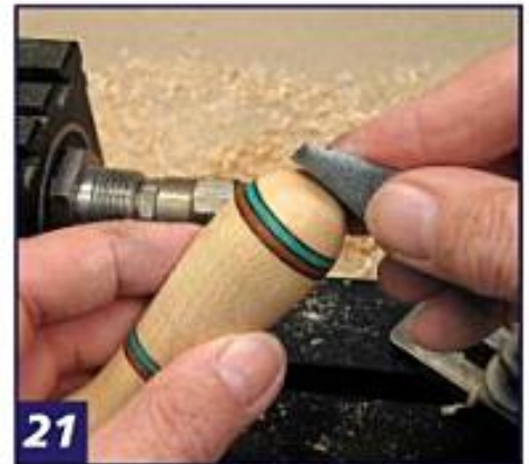
21 Hand sand the parted end to make it smooth.
