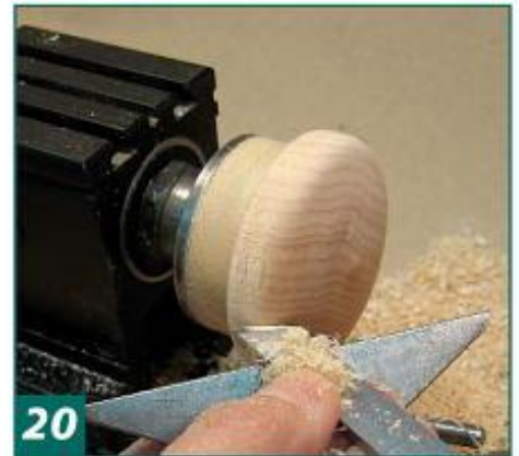
20 A skew lying on its side helps to refine the shapes.
