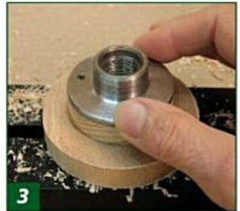
3 Center the faceplate with the glue block onto the workpiece.
