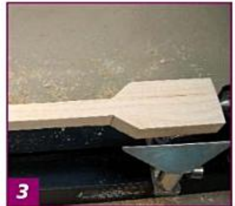
3 Mount the blank between centers with the spatula end centered on the live center point. Keep the speed below 1,800 rpm to start.
