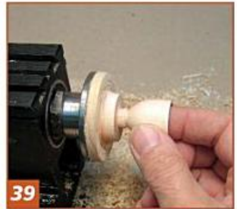
39 Check that the wall thickness is uniform.
