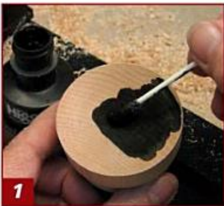
1 Apply black India ink with a Q-tip over the surface before and after you chatter.
