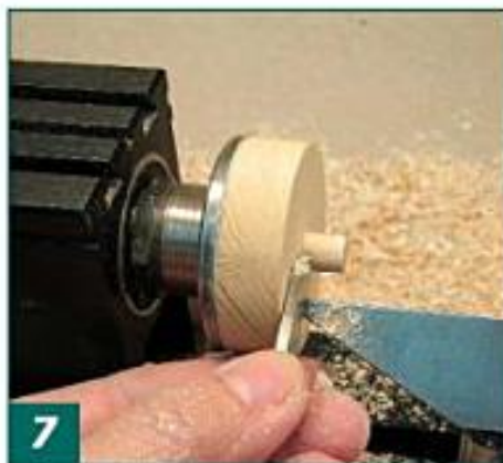
7 Turn down the dowel for a tight press fit in a \frac{1}{16} " hole.
