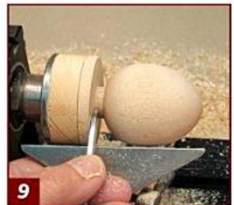
9 Reduce the neck to about \frac{1}{8} " or \frac{3}{16} " diameter. Experiment with different diameters.
