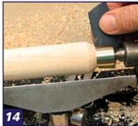
14 Sand the ferrule and polish it with a metal polish if desired. 220-grit sandpaper could be used to achieve a nice satin finish.
