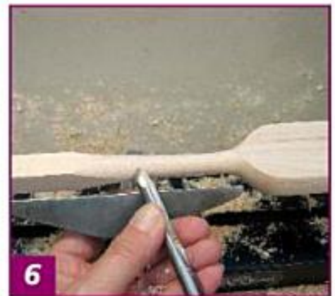
6 Remove the corners and shape the handle as you progress toward the headstock.
