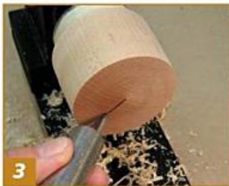
3 You will be moving the chatter tool along this line, with the blade parallel to the line. This is an end view.
