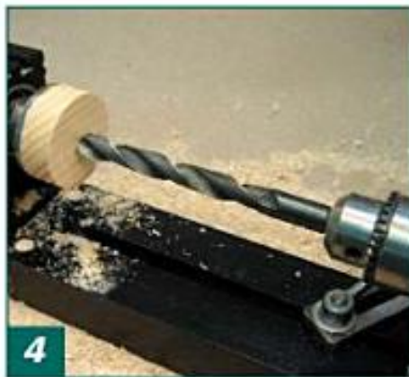
4 Use a \frac{1}{16} " drill bit held in a Jacobs chuck in the tailstock.
