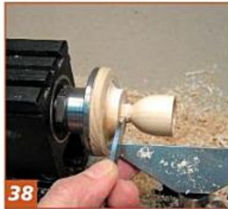
38 Use a parting tool to reduce the neck area as needed.
