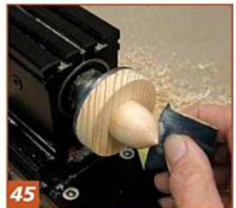
45 Sand smooth, carefully adjusting the final fit of the cap with light sanding.
