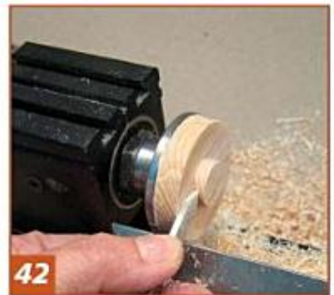
42 Make the tenon about \frac{1}{8} " long with a nice, square shoulder. It should be a snug fit.
