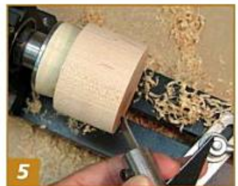
5 This is the view from above. A more closed angle between the face of the tool and the surface of the workpiece will give the tool a better opportunity to chatter.
