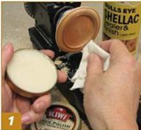
1 Spray shellac and neutral Kiwi wax (for shoes).
