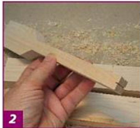
2 Bandsaw to the general shape, cutting the handle to \frac{1}{2} " square with bandsaw cuts for the spur drive.
