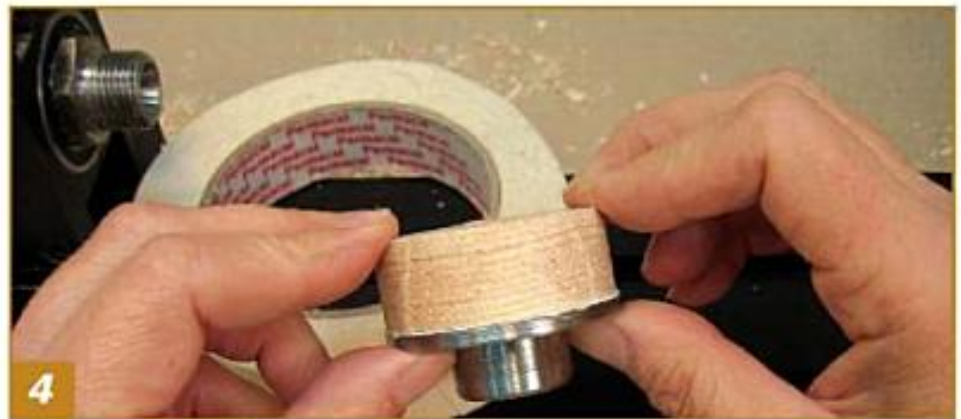
4 Press the glue block onto the tape, and then clamp firmly in a vise for about 15 minutes. This is pressure-sensitive tape and must be clamped for strength. It may be good to reclamp the glue blocks occasionally.
