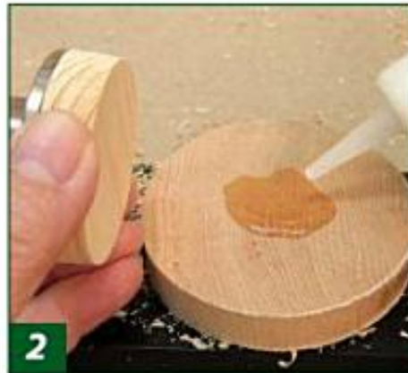
2 Mount the workpiece onto the glue block using CA glue on one side and accelerator on the other side.
