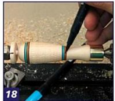
18 Colors will enhance your handles and could be used to more easily distinguish one tool from another.
