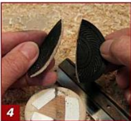
4 Cut in half, the thickness should be about \frac{1}{16} ".
