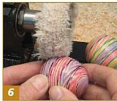
6 Hang on tightly to your workpiece and press it firmly against the spinning buffing wheel. Rotate your workpiece to polish all surfaces.
