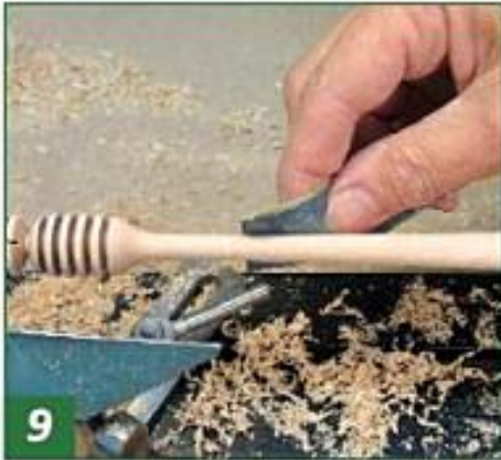
9 Sand the handle after all of the shaping has been done.
