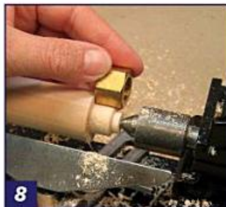
5 With a parting tool, turn a short tenon that will extend through the smaller hole in the compression nut.
