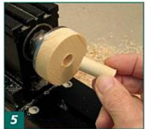
5 Drill a hole about \frac{1}{8} " deep.
