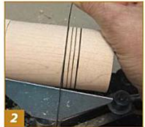
2 The two outer lines have been burned with a heavier gauge wire—about 18g. This wire is stainless steel and won't anneal and break when it gets hot.
