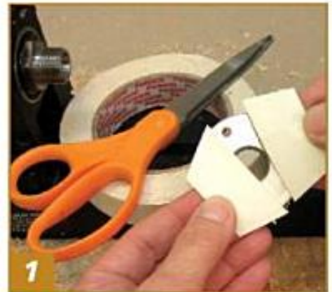
1 Cut pieces of double-faced tape and attach them to your faceplate.
