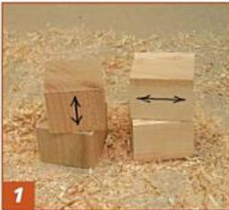
1 Blocks prepared to make two boxes. Blanks for the nuts on the right; blanks for the caps on the left. Arrows indicate grain direction.
