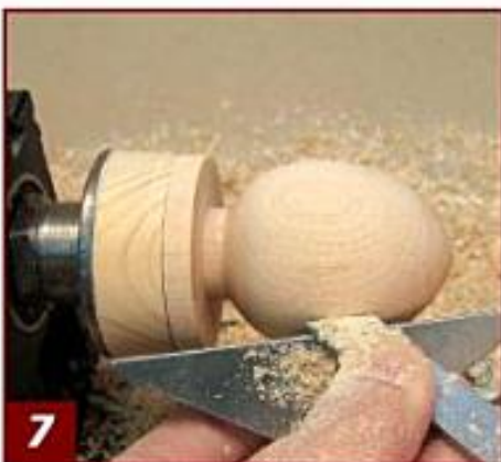
7 A skew lying on its side is useful for lightly refining the shape.
