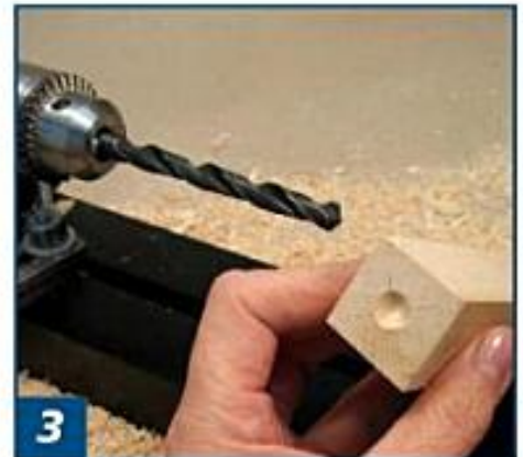
3 Make a starter hole with a hand drill to help center the drill bit, which is held in a Jacobs chuck on the headstock.
