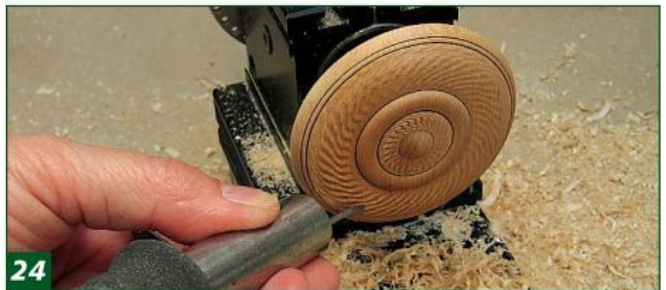
24 Apply a chatter pattern where desired. If you speed up the lathe to about 3,000 rpm and apply more pressure with the chatter tool, you should get an attractive, heavy pattern.
