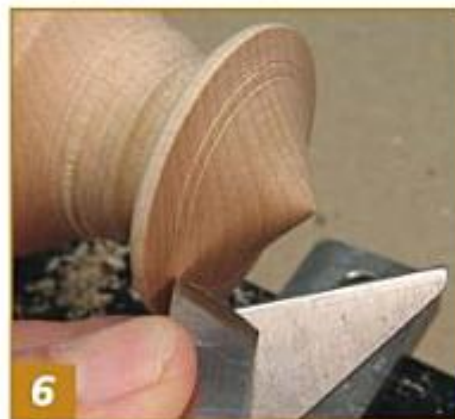
6 If you would like to burn a line on the face of a turning, first make a small groove with the tip of the skew lying flat on the tool rest.
