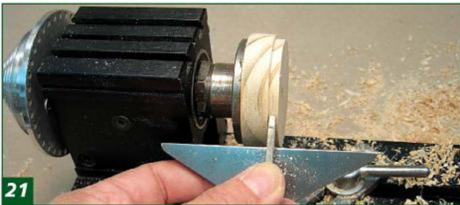
21 Use a wood such as pine as a waste block for reverse chucking the project. The wood you choose for your waste block should be softer than the wood of your project to avoid damage to your project. Using a parting tool, create a tenon almost \frac{1}{4} " long with a good square shoulder for the workpiece to bottom out on.
