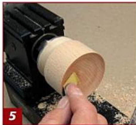
5 Sand it smooth. Since this entire surface is to be chattered, it isn't necessary to use more than one grit.
