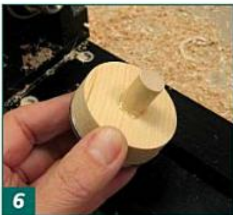
6 Glue in a short section of \frac{1}{8} " hard maple dowel. This will last for many yo-yos.
