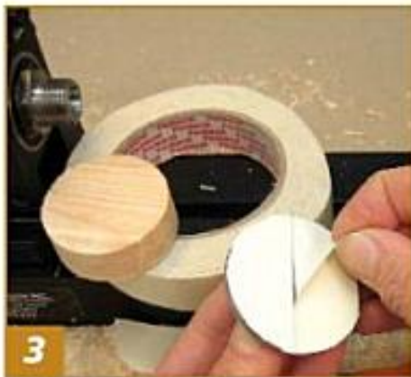
3 Peel off the paper when you are ready to attach a glue block.
