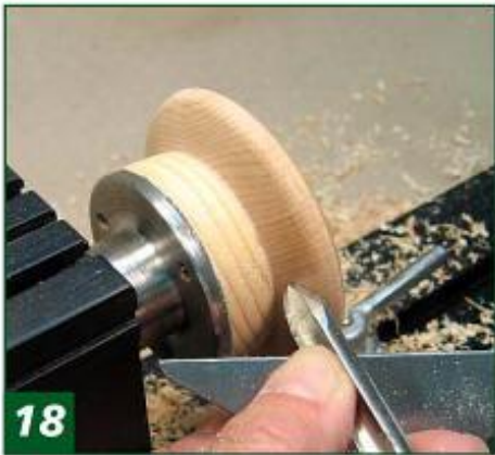
18 Shape the back side of the mirror as far as you can reach.
