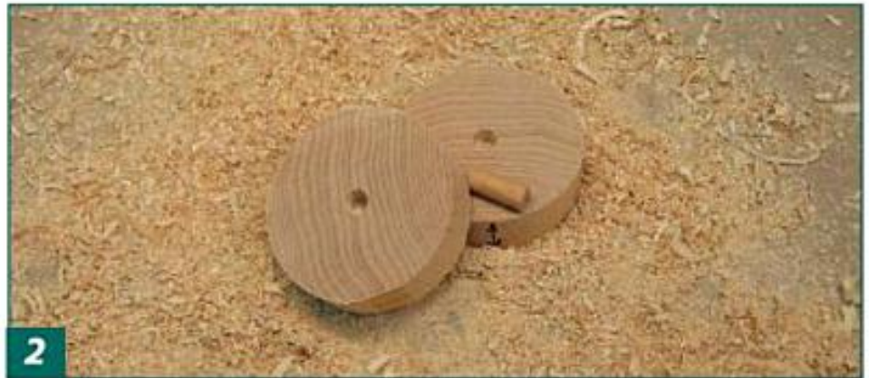
2 Drill \frac{1}{16} "-diameter holes about \frac{1}{8} " deep for the axle. The axle is about \frac{1}{8} " long. These holes must be perpendicular to the faces. Sand the faces smooth to avoid snagging the yo-yo string.
