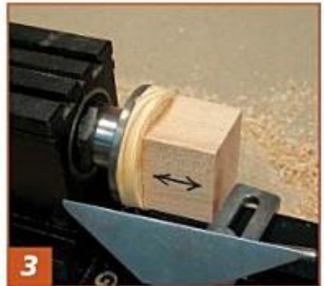
3 Using CA glue, attach the blank for the cap on the target. The grain must be parallel to the lathe bed. (For tips on gluing, see pages 4-5.)
