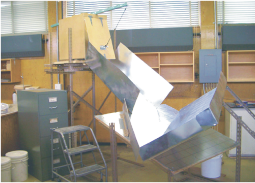
Fig. 10.43. Photograph of the laboratory apparatus at the University of British Columbia used for deflected run-out experiments. (From [273].)
