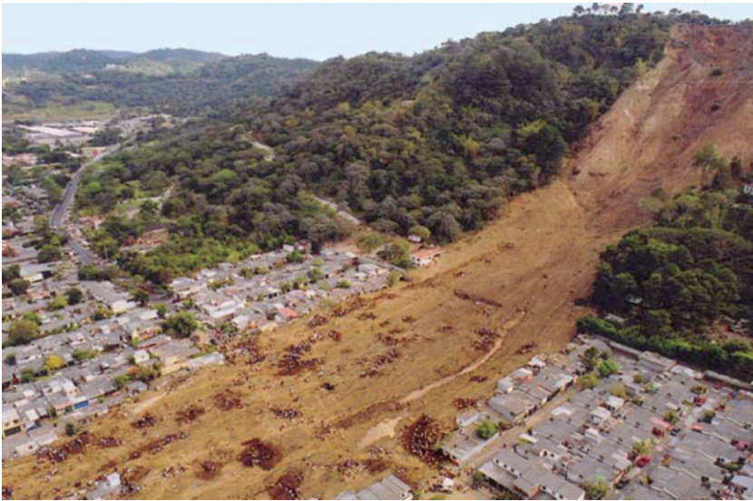
Fig. 1.4. Initiation, channelling, spreading and deposit of a devastating debris slide in Las Colinas (on the outskirts of San Salvador), El Salvador, January 2001. This landslide was induced by an earthquake and may have buried as many as 500 homes [460].
