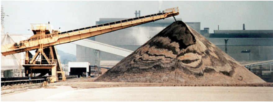
Fig. 1.6. Piling of a mixed bed of granular materials in a cement factory; an example of granular flow and avalanche in process engineering. Different grey scales of the heap correspond to different ingredients of the mixture of the cement. The material is continuously deposited from a quasi-static point source. The material flows rapidly down the faces of the heap in shallow layers. During the downward flux of the fine mixture of granular material, particle segregation according to size, density or resilience takes place. (Courtesy of MVT Materials Handling GmbH, Dillingen.)
