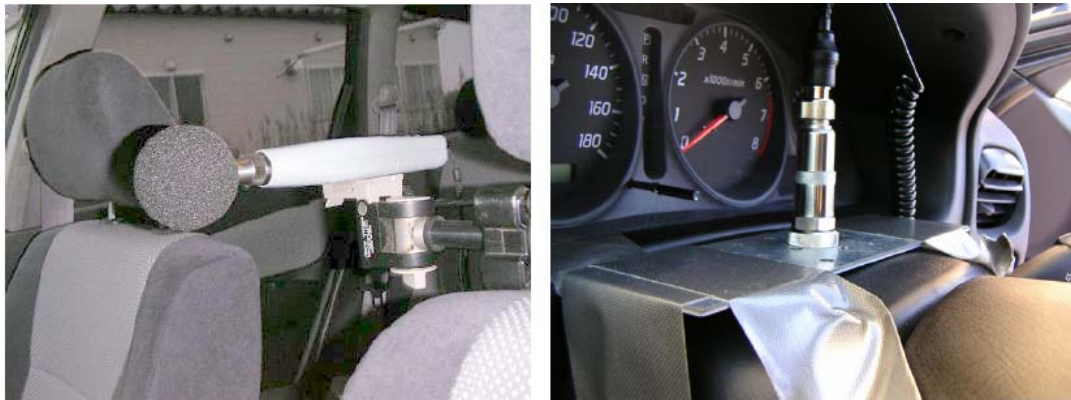
Figure A-4. Setup for Measuring Sound (left) and Vibration (right) (42)
