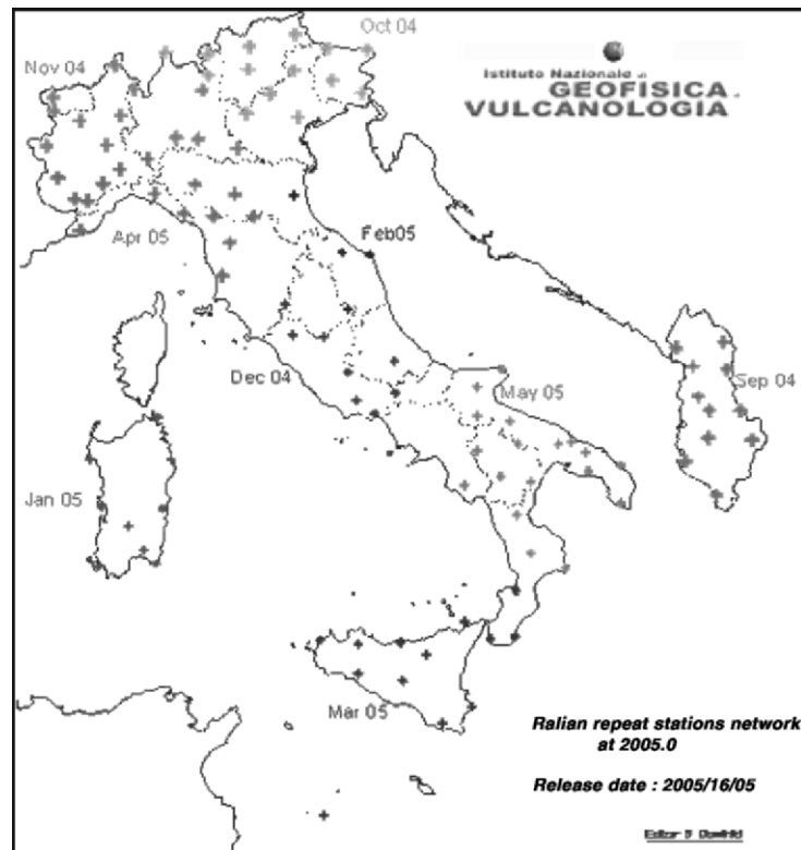
Figure 131. Points of Repeat Magnetic Stations of Italy and Albania and their progress in time so far. Completion of the whole survey (to reach a total of 114 Italian sites + 11 Albanian sites) is foreseen by the end of 2005. During the period of survey also two sites in the seafloor were deployed for magnetic measurements in the framework of the European project GEOSTAR.
