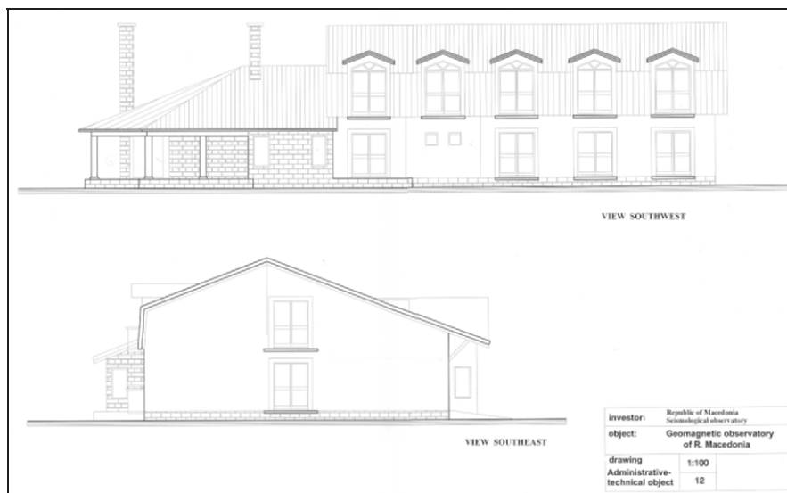
Figure 162. Southwest and southeast view of administrative building.
