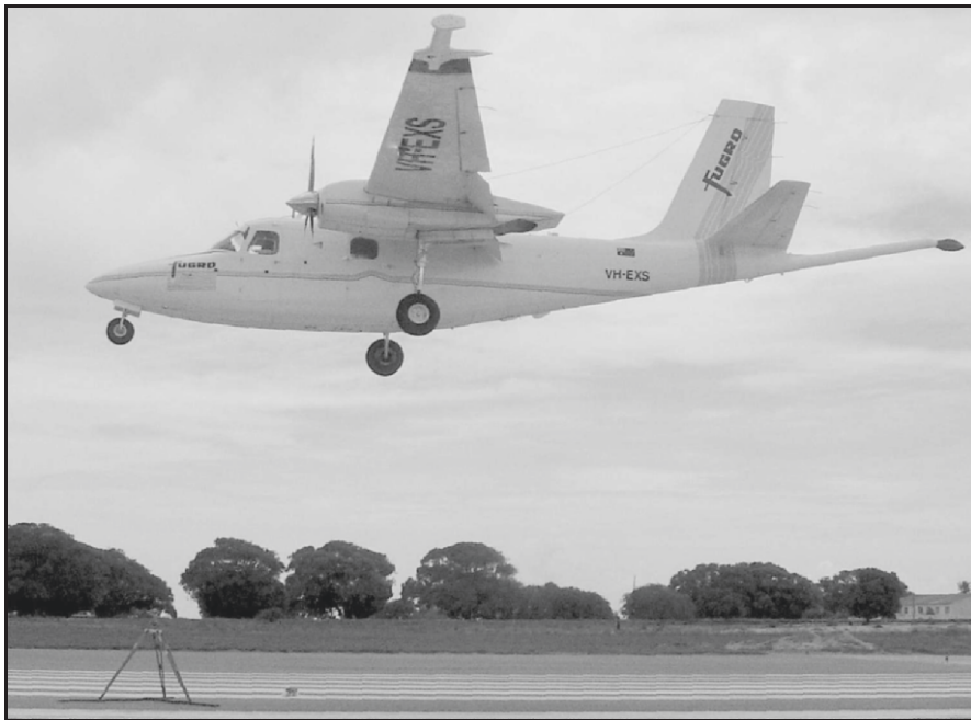
Figure 118. Aircraft landing at the Pemba Airport (Mozambique) while observers are in the process of doing runway azimuth measurements. While the observers could take cover, there was no time to dismantle and evacuate the DIFlux and its tripod, visible at the lower left.
