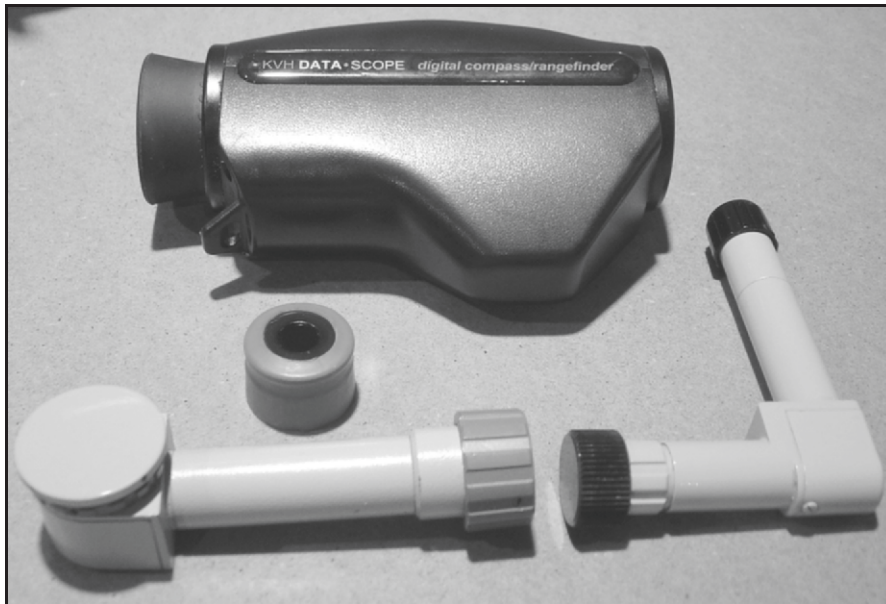
Figure 61. The KVH DATASCOPE Telescope with internal magnetic compass displays the magnetic azimuth of the telescope's optical axis. Also shown are the coudé eyepieces and the solar filter. Essential components for successful sunshots.
