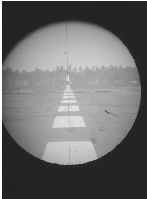
Figure 117. How to sight the runway center line markings through the DIflux telescope. A VOR antenna may be seen aligned with the runway at its terminus.
