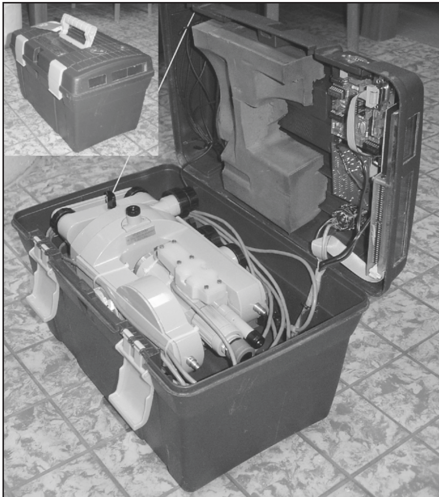
Figure 62. The ZEISS 010B DIflux with FLM3/A fluxgate electronics and GPS receiver.
