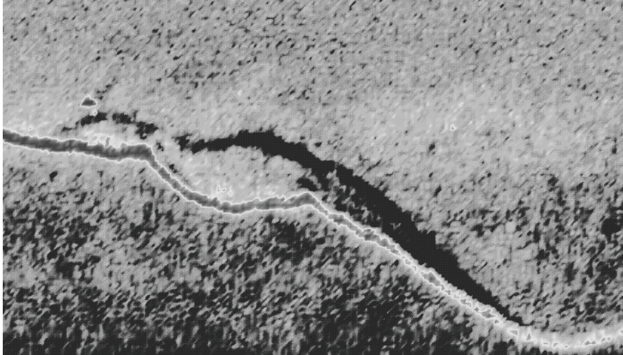
Figure 7-5. Convergent front on the continental shelf detected by airborne radar. This X-band radar image (~2.25x1.25 km) was one of several collected by Farid Askari (NRL) near Cape Hatteras, NC during the first High Resolution Remote Sensing Experiment. (This image is from the public domain of the Naval Research Laboratory Website http://rsd-www.nrl.navy.mil/7250/ )
