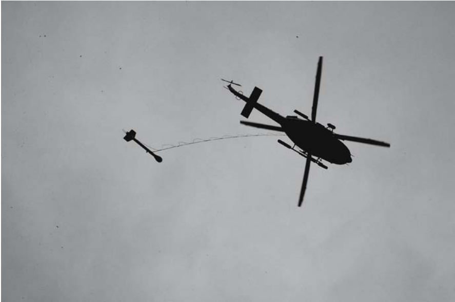
Fig. 3.2. Photograph of an helicopter borne survey in action. The sensor of the magnetic instrumentation is kept at secure distance from the helicopter to avoid artificial magnetic effects (courtesy M. Chiappini)
