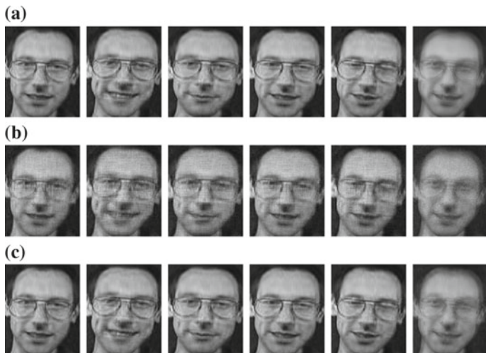
Fig. 3.2 Reconstructed images and ( robust ) mean images: a outlier-free reconstruction by MPCA, b MPCA, c RMPCA. In each row, the left five images are the reconstructed ones, and the rightmost image is the mean one. © 2009 IEEE
