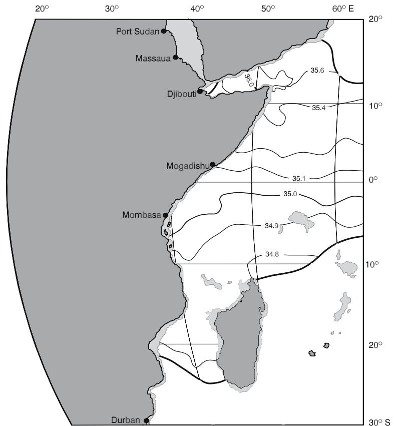
Figure 2.18. The distribution of salinity in the salinity maximum core layer formed at intermediate depths in the South West Indian Ocean by Red Sea Water 84 . This core layer is found at depths of 1000 to 1100 m in this ocean region. The heavy line shows the southern limit to the influence of this particular water mass, much farther poleward in the Mozambique Channel than elsewhere in this ocean region.
