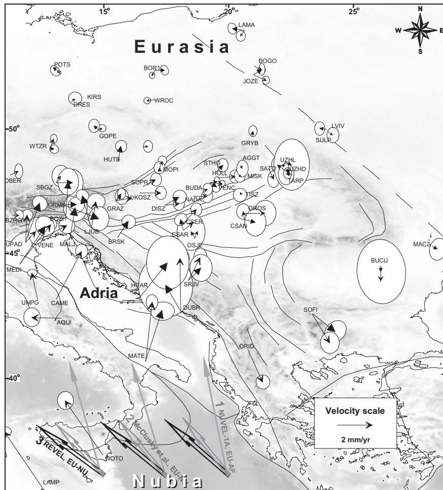
Figure 2. Velocities of GPS stations in Central Europe from continuous and epoch-type observations together with their 95% confidence ellipses relative to stable Eurasia. Plate motion of Nubia with reference to Eurasia 1: NUVEL-1A Africa-Eurasia (geophysical data over 3 Myr), after DeMets et al., 1994; 2: Nubia-Eurasia (recent space geodetic data) after McClusky et al., 2003; 3: REVEL IT97-2000 Nubia-Eurasia (recent space geodetic data); after Sella et al., 2002. Figures 3 and 4 show interpolated velocity fields derived from the velocities shown here.
