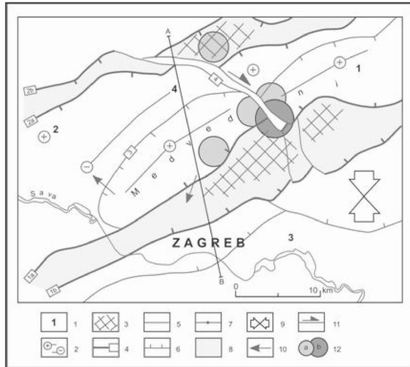
Figure 2. Geologic structure of Mount Medvednica: 1 – structures, 2 – axes of maximal and minimal Bouguer anomalies, 3 – zones of larger gravity gradients, 4 – Medvednica-Zumberak fault (1a – Zagreb fault), 5 – Medvednica faults, 6 – reverse faults, 7 – faults with unknown direction, 8 – fault zones, 9 – orientation of maximal compression stress, 10 – direction of subsurface motions of Medvednica, 11 – fault with horizontal motion, 12 – Epicentres of the strongest earthquakes.
