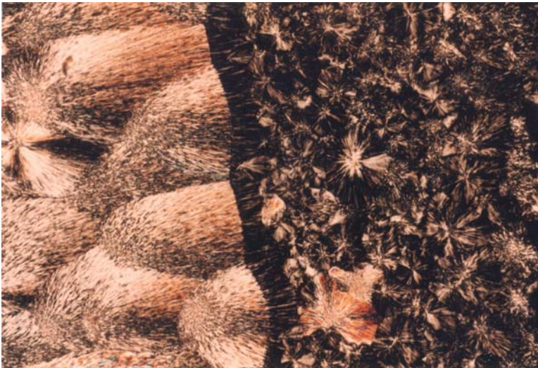
Fig. 1.29 Morphology at the crystallization zone of an iPP, if this zone has proceeded over a considerable distance into the sample. The fine grained structure on the right is caused by the final quench. For conclusions see the text. Ewa Ratajski, unpublished
