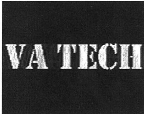
Figure 10-9f) Digital reconstruction using the proposed chirp-Gaussian function given by Eq. (10-15)
