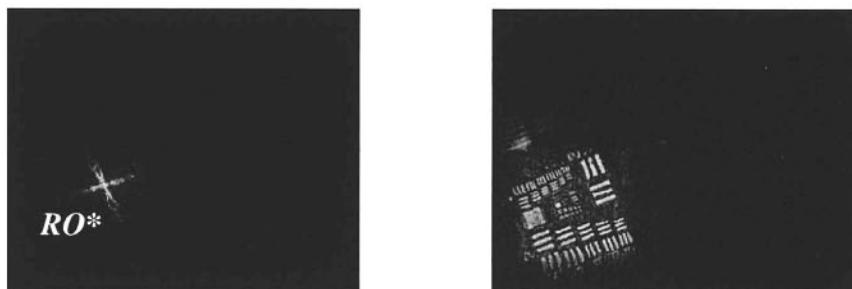
Figure 4-7. Role of filtering out  $RO^*$ : delineating the zone around the spot attributed to  $RO^*$  permits reconstructing only the virtual image (Cucho, 2000).
