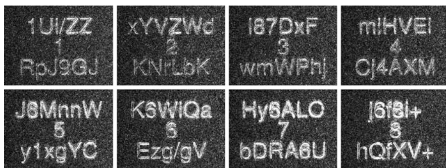
Fig. 45 Reconstruction of eight two-dimensional images which were inscribed at the same spot of a thick sample of material 18 under angle intervals of 1^\circ each. The object beam had a diameter of about 1 mm in the sample. Writing was performed with a wavelength of 514 nm, ss-polarization, and a total fluence of 2 \text{ J cm}^{-2} per hologram. (Reprinted with permission from [79]. Copyright 2009 SPIE)
