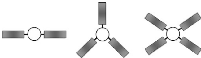
Fig. 8 Schematic structure of different topologies of photoaddressable azobenzene containing molecular glasses with two, three, and four azobenzene moieties; ( open circles ) core; ( filled rectangles ) azobenzene chromophore units
