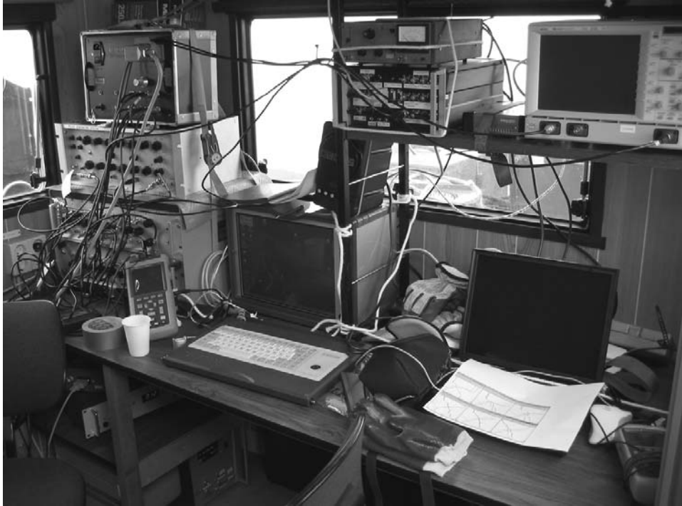
Figure 11.14. The data acquisition system onboard HMS Fårösund .
