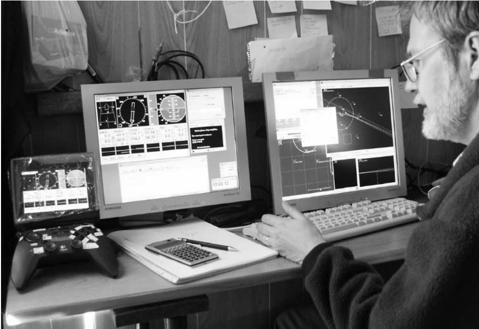
Figure 11.12. Interface designed to operate the ROV and parametric sonar for the multiple-aspect measurements.
