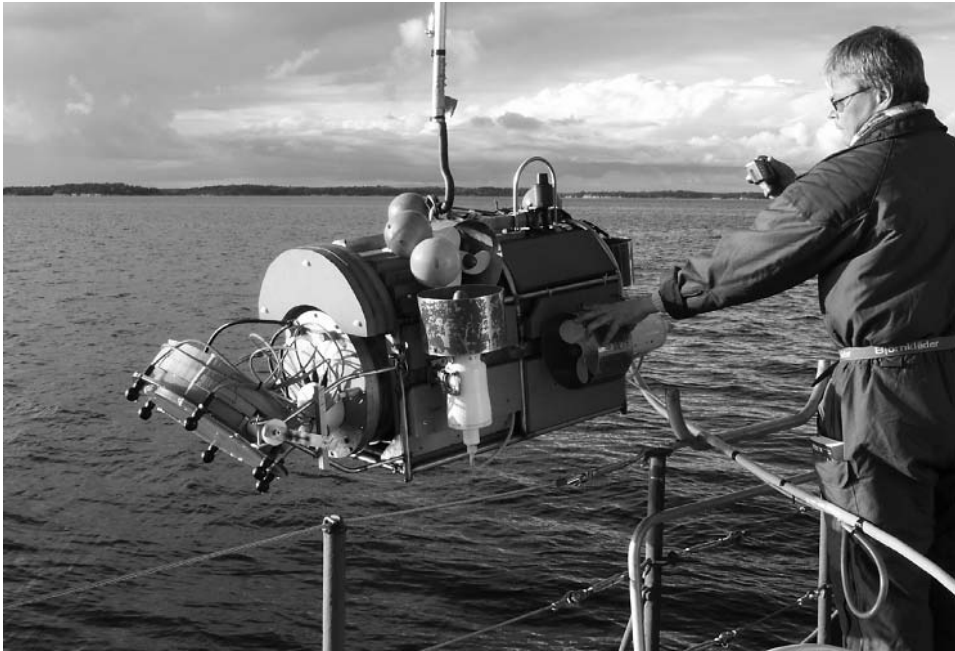
Figure 11.11. The ROV developed by FOI called Plums (platform for underwater measurement systems) equipped with the TOPAS 120 parametric sonar.
