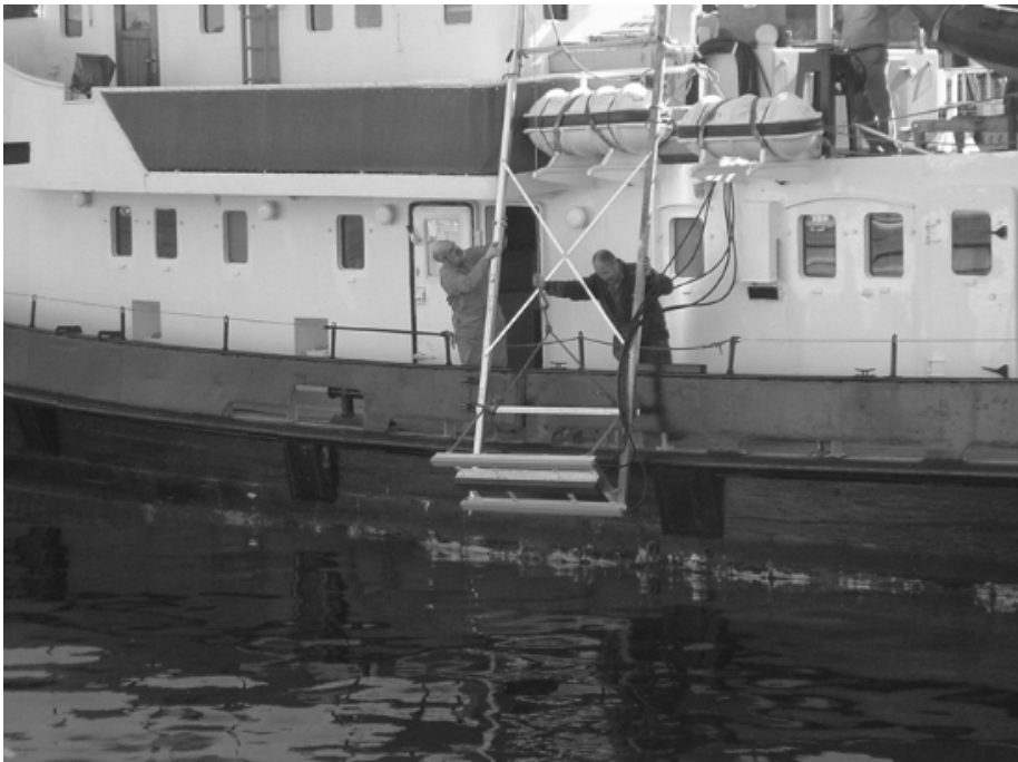
Figure 11.8. The parametric side-scan sonar prototype mounted on the frame is here ready for launch.
