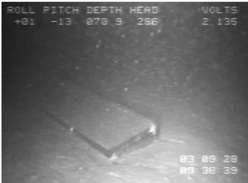
Figure 11.6. Two different views of the semi-buried box, the target for multiple-aspect measurements. The size of the box is approximately 1.3 \times 0.3 \times 0.3 m.
