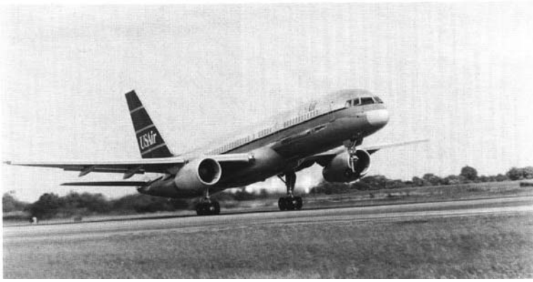
Fig. 11.6 Rolls-Royce RB211-525E4 turbo-fan engines, installed in a Boeing 757 (courtesy of Rolls-Royce plc)
