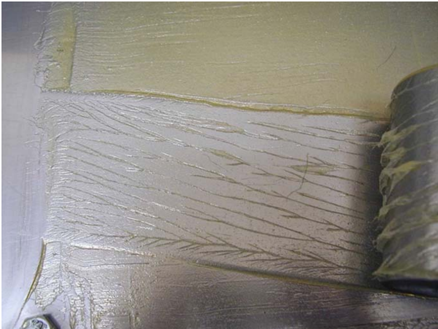
Fig. 14.5 The filament/fibrillar structure of a grease film in the track of a roller
