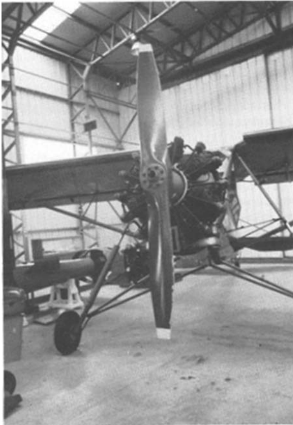
Fig. 11.3 Jacobs radial engine, installed in a Morane-Saulnier MS.505 (courtesy of Scottish Museum of Flight)
