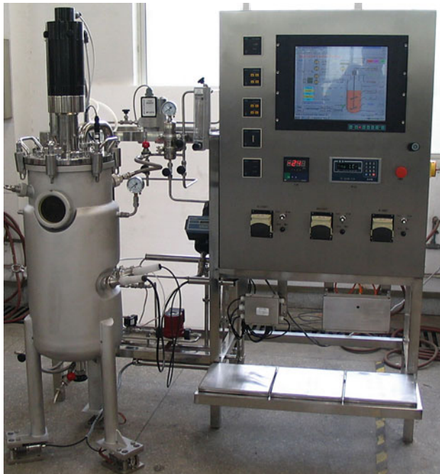
Fig. 5 The novel fermentation apparatus manufactured by Shanghai Guo Qiang Company Ltd for Biochemical Engineering Equipments
