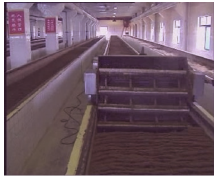
Fig. 18 The machine upturner automatically turns cu pei in acetic acid fermentation pool
