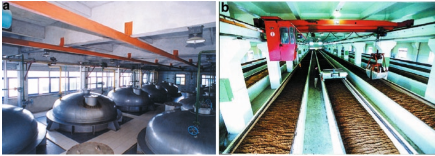
Fig. 17a,b Vinegar production with large-scale alcohol fermenters (a) and acetic acid fermentation pools (b)
