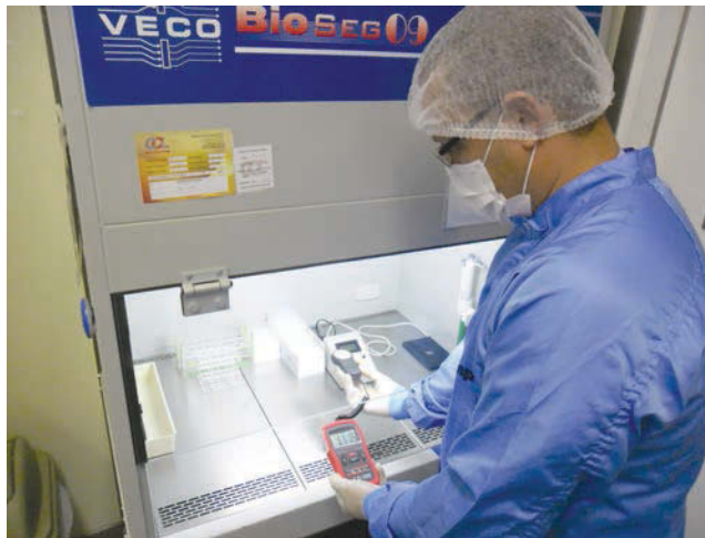
Figure 16.21 Light intensity measurement. Photograph showing a Class II biosafety cabinet being checked with a light meter. (Courtesy of Androfert, Campinas, Brazil.)
