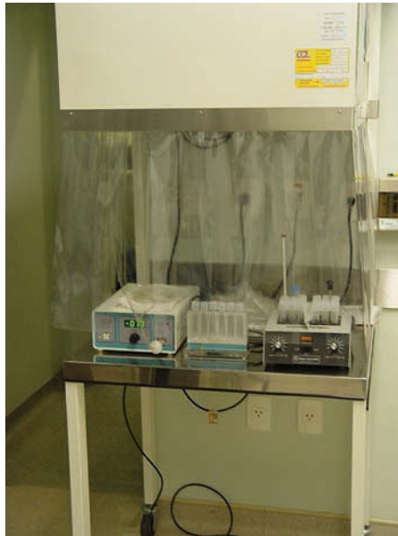
Figure 26.11 Cabinet in which tubes to collect follicular fluid are handled during oocyte pick-up. A ceiling-mounted high efficiency particulate air (HEPA) filtration system provides vertical unidirectional airflow to the work area.
