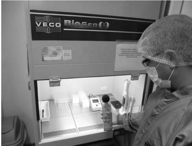
Figure 16.22 (See color insert.) Photograph showing a Class II biosafety cabinet being checked with a sound level meter. (Courtesy of Androfert, Campinas, Brazil.)
