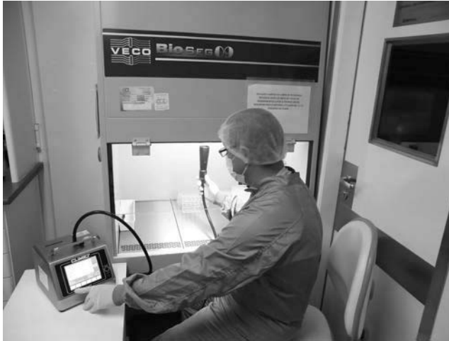
Figure 16.5 (See color insert.) Particle counting in Class II biosafety cabinet. (Courtesy of Androfert, Campinas, Brazil.)
