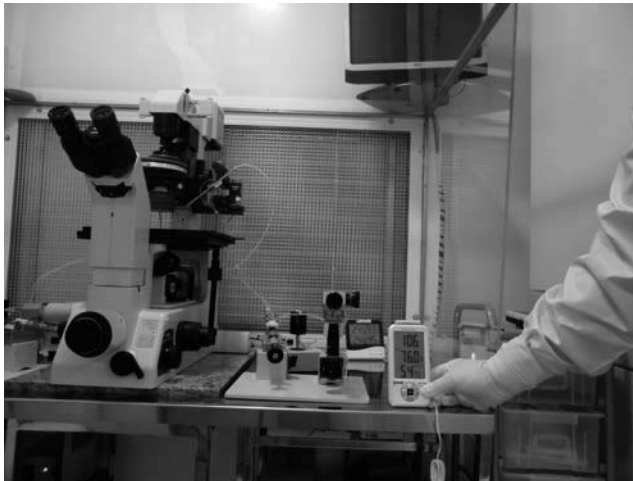
Figure 16.19 Ambient humidity and temperature measurement. Photograph showing an engineer using a thermo hygrometer to monitor air humidity and temperature in the clean room IVF laboratory. (Courtesy of Androfert, Campinas, Brazil.)
