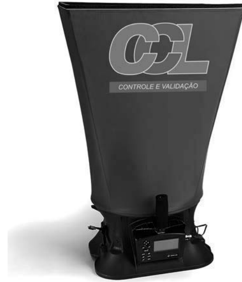
Figure 16.6 Balometer is an electronic flow meter custom designed to measure the air volume supplied by diffusers and grills.
