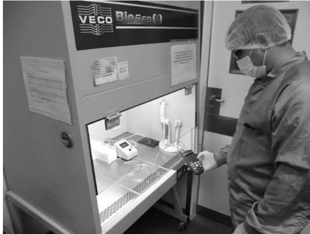
Figure 16.14 Air pressure differential. Photograph showing a Class II biosafety cabinet being checked with micromanometer. (Courtesy of Androfert, Campinas, Brazil.)
