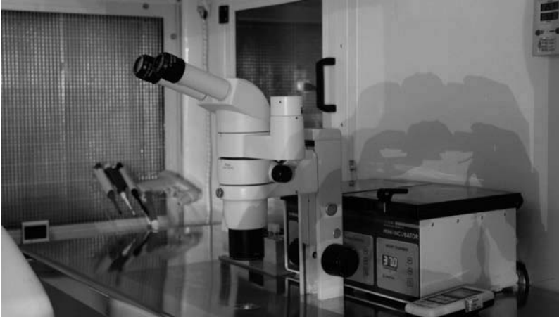
Figure 26.5 (See color insert.) Overview of a workstation for handling oocytes and embryos. A wall-mounted frame with a terminal high efficiency particulate air (HEPA) filter supplies unidirectional airflow within the work area.
