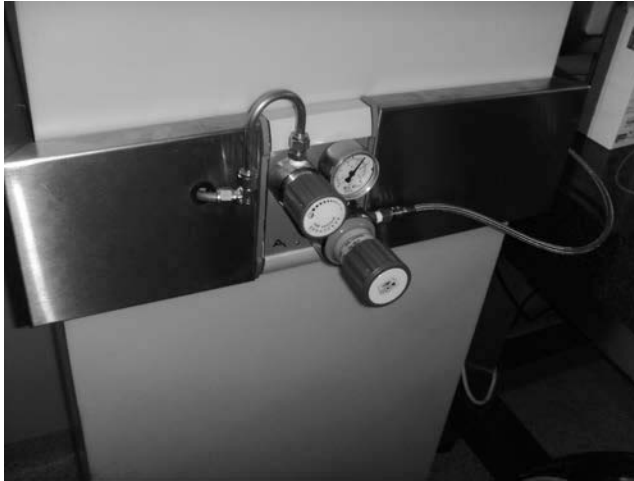
Figure 9.9 Inside the IVF lab: second regulator connecting to the incubator. (Courtesy of Giles Palmer, London Womens Clinic, UK.)
