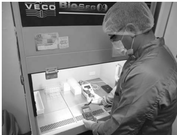
Figure 16.21 (See color insert.) Light intensity measurement. Photograph showing a Class II biosafety cabinet being checked with a light meter. (Courtesy of Androfert, Campinas, Brazil.)
