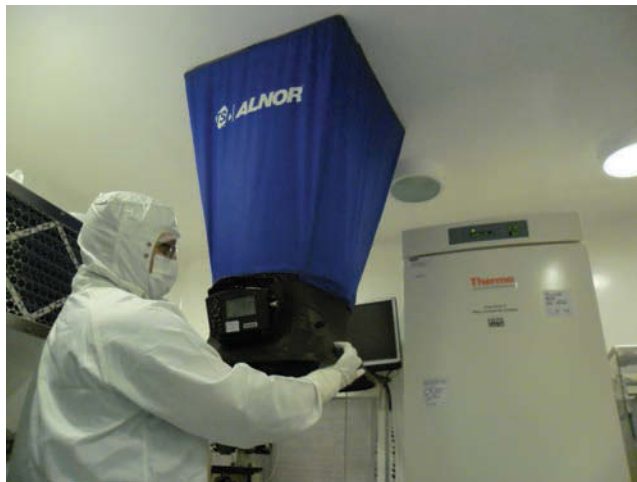
Figure 16.7 Air flow volume and air speed assessment. Photograph showing an engineer testing an air diffuser with a balometer in the clean room IVF laboratory. (Courtesy of Androfert, Campinas, Brazil.)
