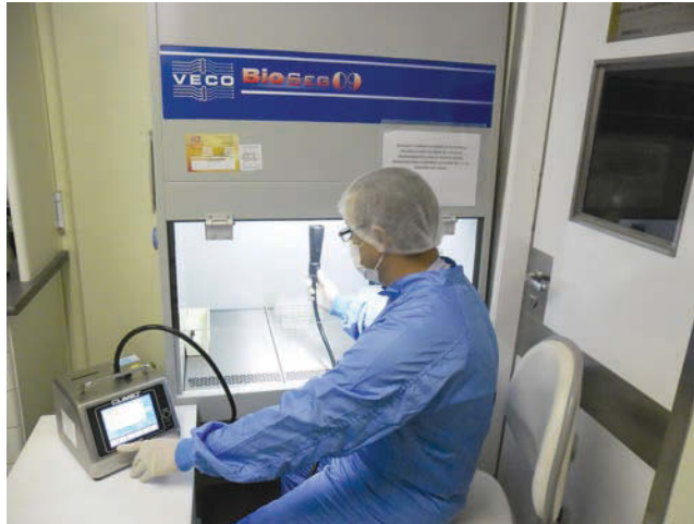
Figure 16.5 Particle counting in Class II biosafety cabinet. (Courtesy of Androfert, Campinas, Brazil.)
