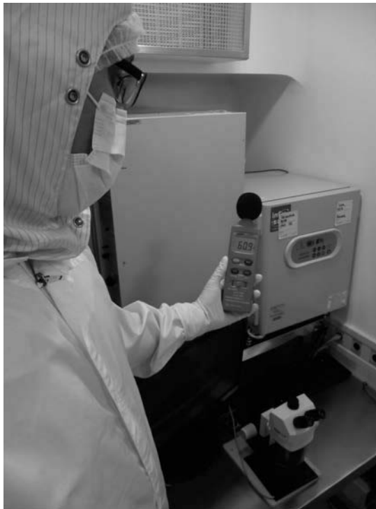
Figure 16.23 Sound level measurement. Photograph showing an engineer using a sound level meter to monitor noise level in the clean room IVF laboratory. (Courtesy of Androfert, Campinas, Brazil.)
