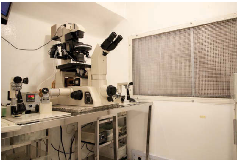
Figure 26.4 Overview of a workstation for micromanipulation of oocytes, sperm, and embryos. A wall-mounted frame with a terminal high efficiency particulate air (HEPA) filter supplies unidirectional airflow within the work area.
