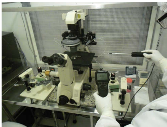
Figure 16.10 Air flow volume and air speed assessment. Photograph illustrating an engineer checking air flow volume and air speed of an unidirectional air flow workstation with a thermo-anemometer. (Courtesy of Androfert, Campinas, Brazil.)
