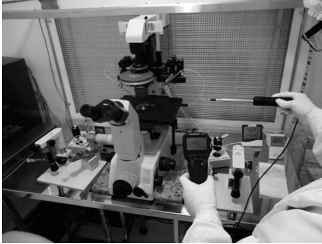
Figure 16.10 (See color insert.) Air flow volume and air speed assessment. Photograph illustrating an engineer checking air flow volume and air speed of an unidirectional air flow workstation with a thermo-anemometer. (Courtesy of Androfert, Campinas, Brazil.)
