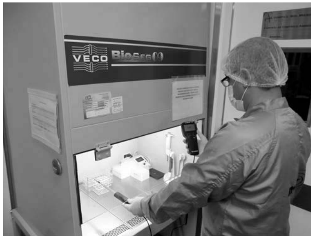
Figure 16.9 (See color insert.) Air flow volume and air speed assessment. Photograph showing a Class II biosafety cabinet being checked for air flow volume and speed with a thermo-anemometer. (Courtesy of Androfert, Campinas, Brazil.)
