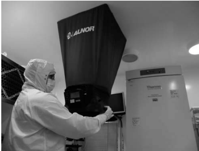
Figure 16.7 (See color insert.) Air flow volume and air speed assessment. Photograph showing an engineer testing an air diffuser with a balometer in the clean room IVF laboratory. (Courtesy of Androfert, Campinas, Brazil.)
