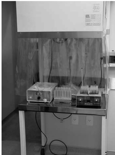
Figure 26.11 (See color insert.) Cabinet in which tubes to collect follicular fluid are handled during oocyte pick-up. A ceiling-mounted high efficiency particulate air (HEPA) filtration system provides vertical unidirectional airflow to the work area.
