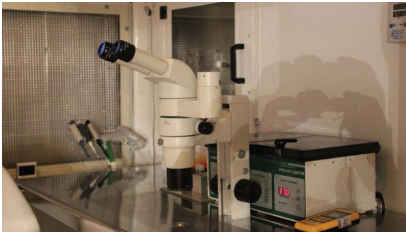
Figure 26.5 Overview of a workstation for handling oocytes and embryos. A wall-mounted frame with a terminal high efficiency particulate air (HEPA) filter supplies unidirectional airflow within the work area.
