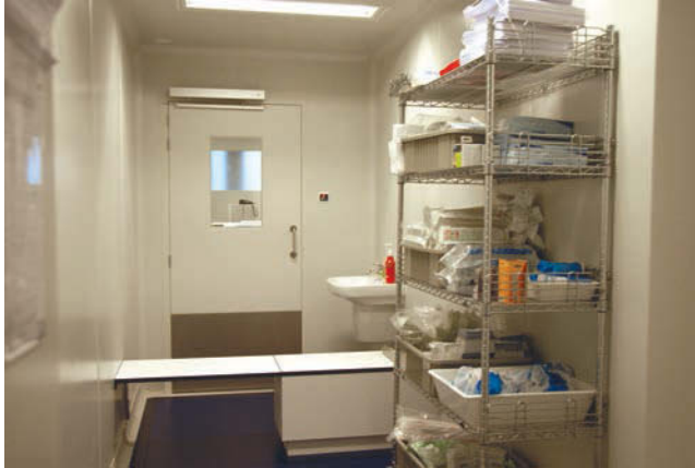
Figure 14.2 Entrance room into IVF clean room facility using a cross bench. Staff should sit on the bench to remove their shoes, move the legs over the bench and put on the clean room shoes. Staff can stand up and move into the clean room by stepping on a sticky clean room mat. Hands should be disinfected after changing of shoes and before entrance into the IVF clean room facility.
