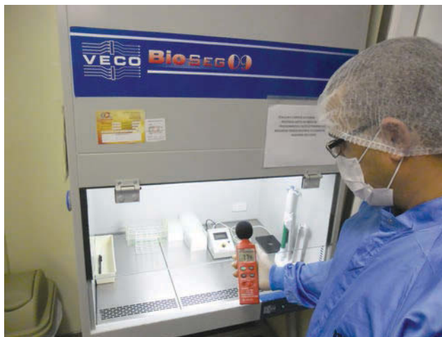
Figure 16.22 Photograph showing a Class II biosafety cabinet being checked with a sound level meter. (Courtesy of Androfert, Campinas, Brazil.)
