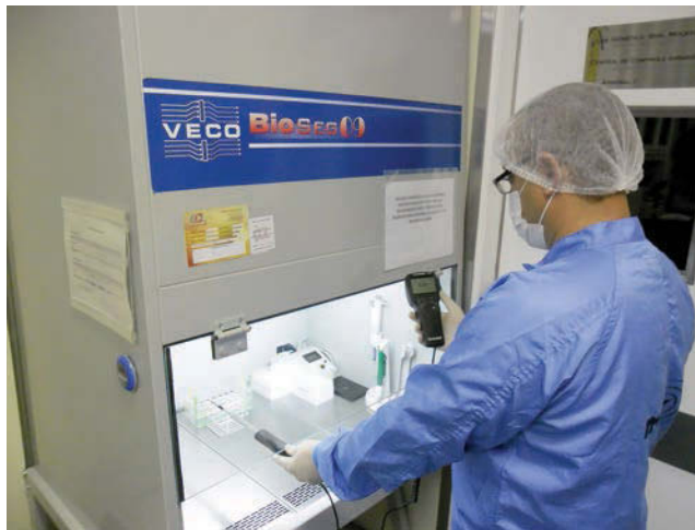
Figure 16.9 Air flow volume and air speed assessment. Photograph showing a Class II biosafety cabinet being checked for air flow volume and speed with a thermo-anemometer. (Courtesy of Androfert, Campinas, Brazil.)
