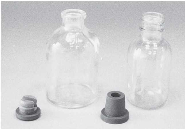
Fig. 16. Culture bottles that this author uses. Left: Wheaton glass serum bottle (Lawson Mardon Inc., Mays Landing, NJ). 50-mL size (#223745); autoclave before use. Between three and five embryos can be cultured in a bottle. At least 4.5 mL of culture medium is needed to maintain enough depth, 4–5 mm. Right: Wheaton polyethylene terephthalate bottle, 45-mL size (Wheaton, #221133); gas sterilization is ideal, although rinsing the inside with alcohol seems to be good enough to prevent bacterial growth together with antibiotics in the culture medium. As many as three embryos can be cultured in a bottle. A rubber stopper of an appropriate size is recommended rather than the plastic screw cap that comes with the bottle, because it takes less time to close the bottle after gassing.
