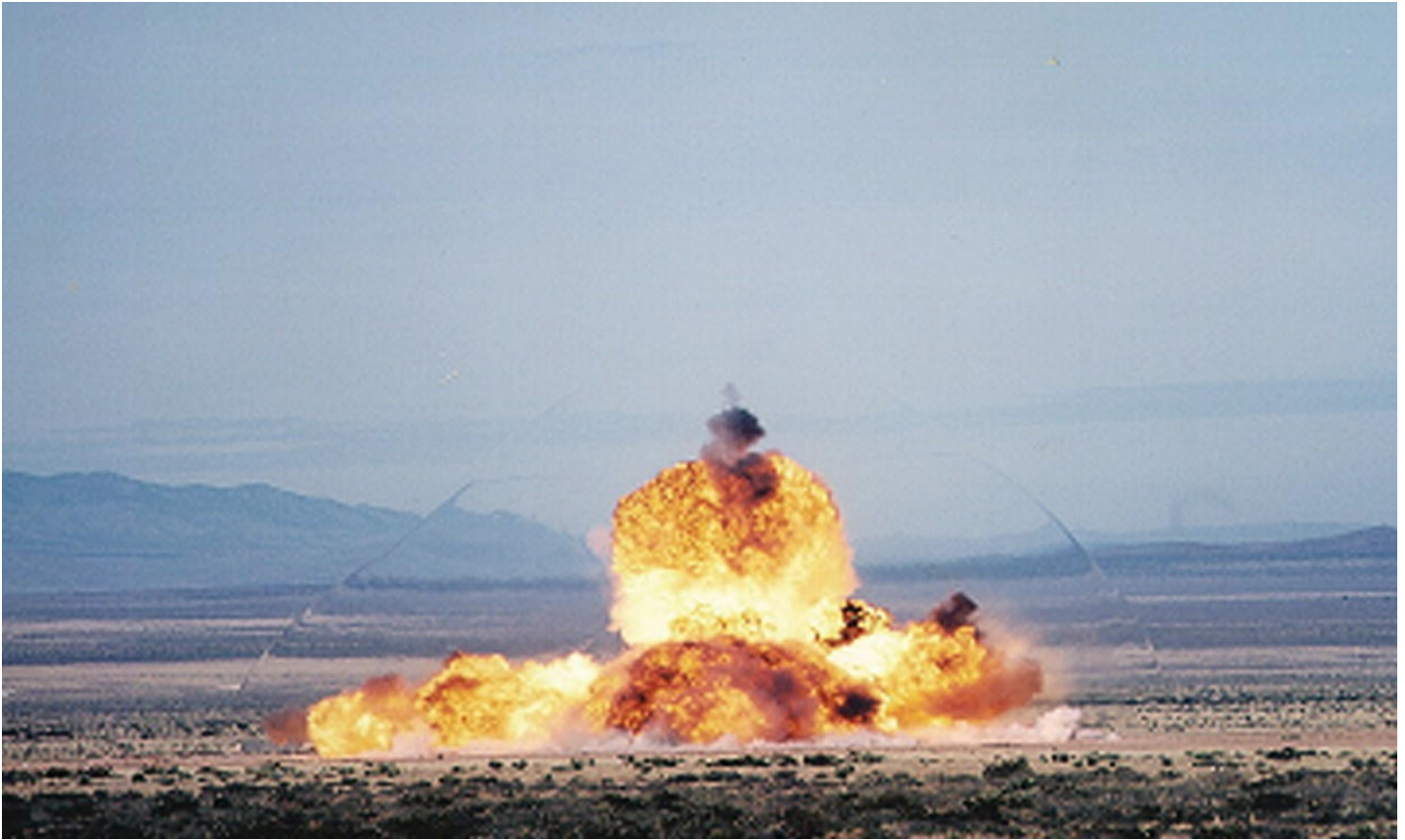
Figure 5.1 Explosion of 20,000 pounds of Composition C-4 inside a small truck. Note that the shock wave is visible due to its extreme effect on the refractive index of the surrounding air. The “thermal event” occurs within the volume defined by the shock wave.
