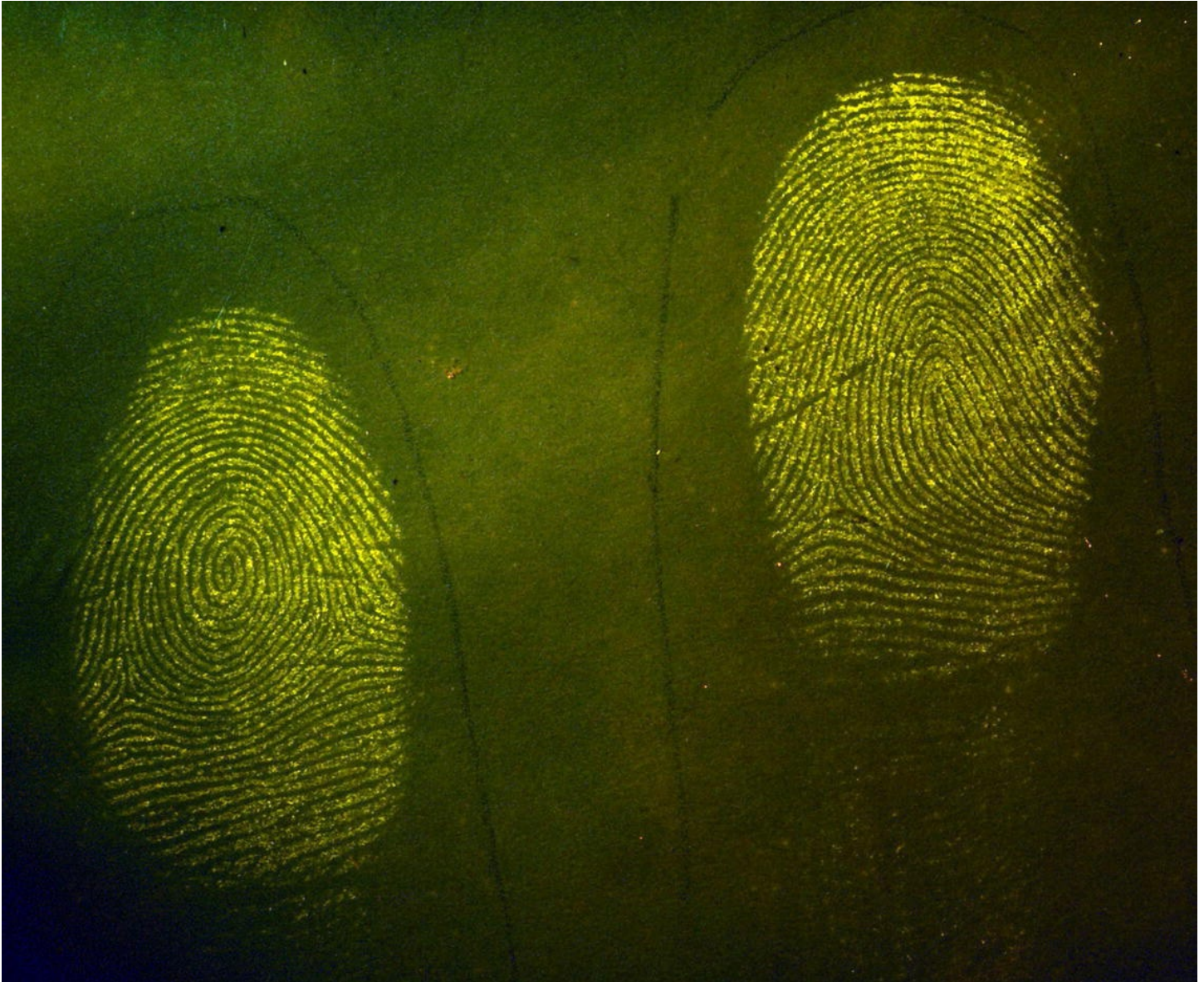
Figure 9.14 Fingerprints on white copy paper developed with Nile blue, viewed through a 550 nm barrier filter with illumination at 505 nm
