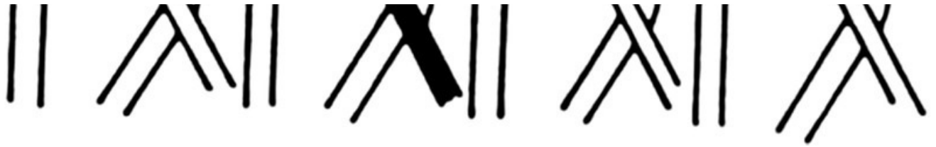
Figure 2.11 The basic pattern of warp knitting has yarns zigzag lengthwise along the fabric, with each loop securing a loop of an adjacent strand from the previous course.
