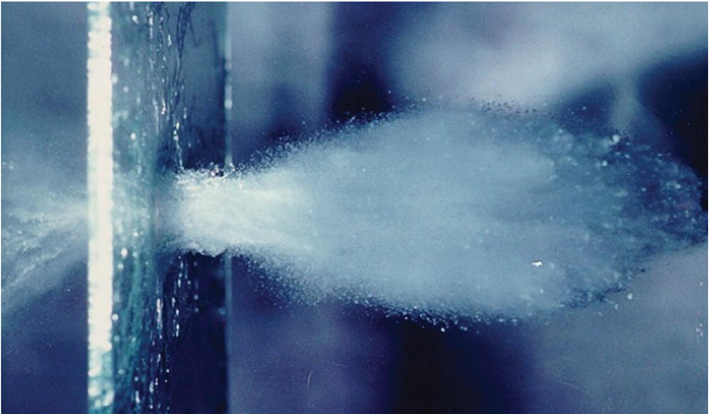
Figure 6.3 High speed photography of a bullet penetrating a glass pane
