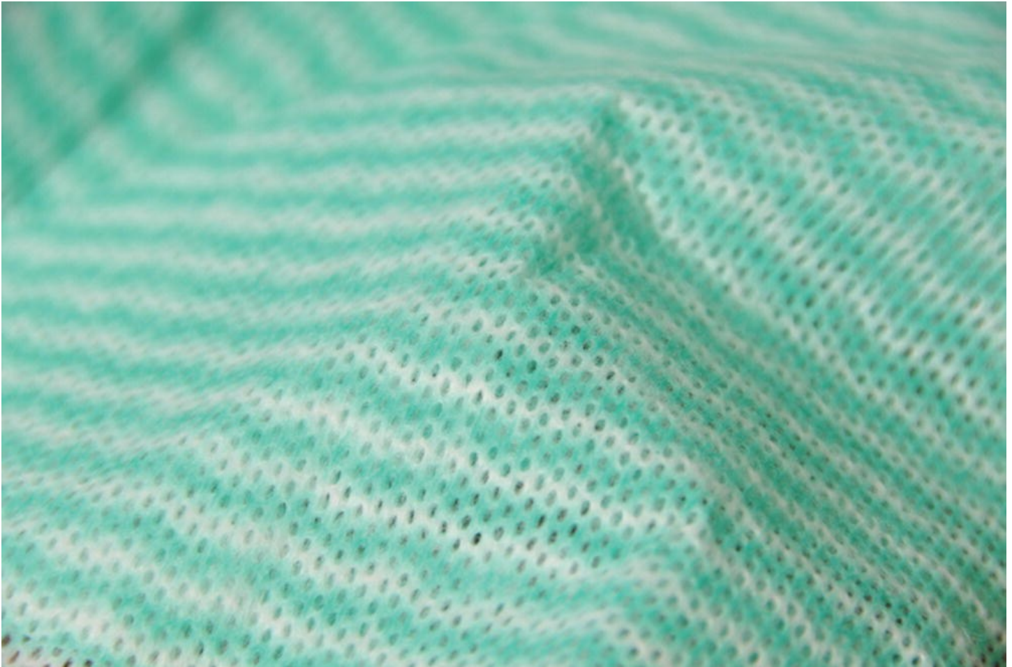
Figure 2.12 Non-woven fabrics are made by any method that can entangle the fibers and have them stay together. In this image of a disposable wipe, the individual fibers have been entangled by water and then pressed together by passing the fibers through rollers. The rollers have small studs which press the holes into the fabric, giving it more surface area and making the fabric more absorbent
