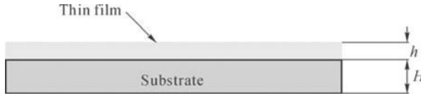
Fig. 6.7 Schematic of ferroelectric thin film and substrate system
