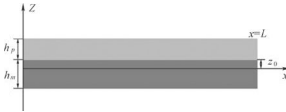
Fig. 8.23 Bilayer of magnetostrictive and piezoelectric components. The middle plane is defined as z=0 and the interface of the bilayer is located at z=z_0
