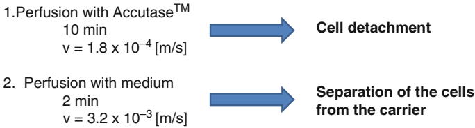
Fig. 11 Harvesting of hMSC-TERT in fixed-bed reactors based on non-porous borosilicate glass spheres
