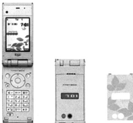
Figure 6.4 FOMA(TM) N701iECO phone made of PLA bioplastics reinforced with kenaf fibres developed by NEC, UNITIKA and NTTDoCoMo © Paul Fowler [50]
