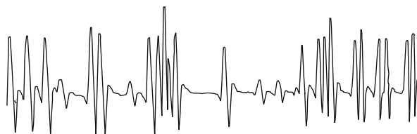
Fig. 11.63. Derivative saturation spectrum of the iodine transition B^3\Pi_u ( v' = 58, J' = 99 ) \leftarrow X^1\Sigma_g ( v'' = 1, J'' = 98 ) with 21 hfs components
