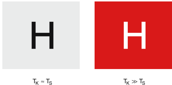
Fig. 3.2. The letter H mill-cut into a graphite cube appears completely black at temperature T_k < T_s = temperature of the surrounding, but appears bright for T_k \gg T_s
