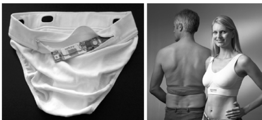
Figure 6.1-13. Flexible ECG monitoring device appropriate for integration into underwear (left), textile belts or bras (right). (Copyright Philips Research Aachen, modified and reprinted by permission.)
