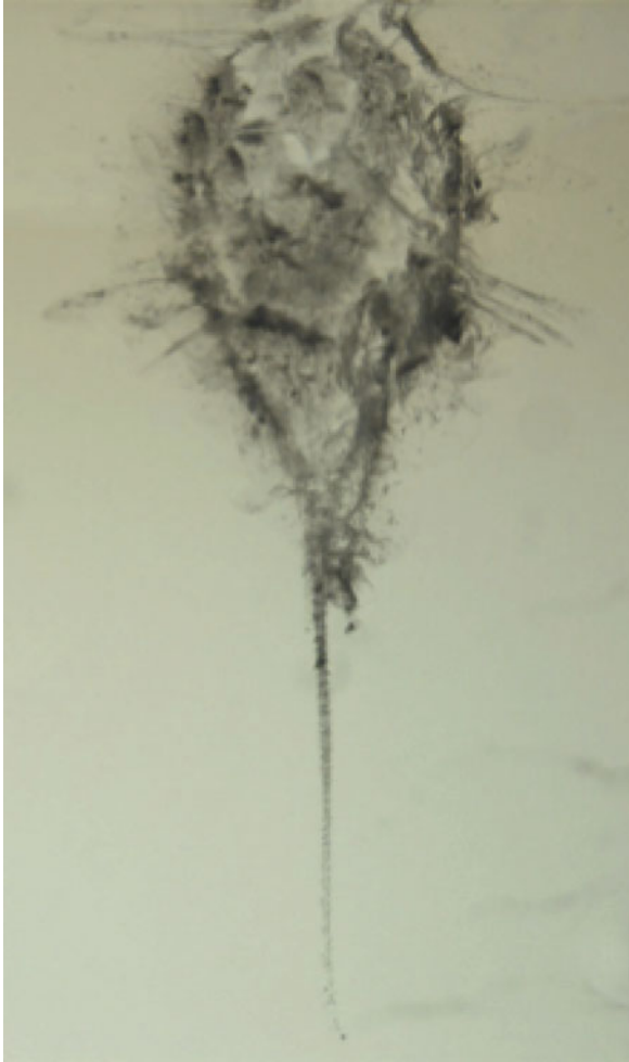
Fig. 5 Example of a track (C054-T3) in the Wild 2 aerogel collector. showing bulbous upper cavity with narrow tracks of terminal grains branching from it
