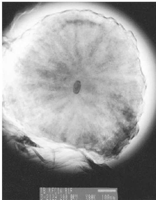
Fig. 10 TEM micrograph of an ultrathin section of an onion-type circumstellar graphite grain. Included in the graphite grain is a TiC subgrain. Figure courtesy of T.J. Bernatowicz
