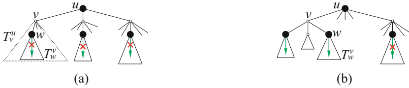
Fig. 5. (a) A (T, I) -rigid token on u , and (b) a (T, I) -movable token on u
