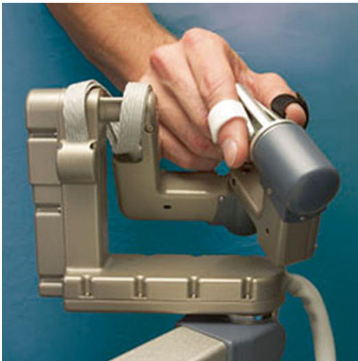
Fig. 14.4 The daVinci master control interface used to remotely manipulate the wristed robotic instruments tip (From Freschi et al. [22])
