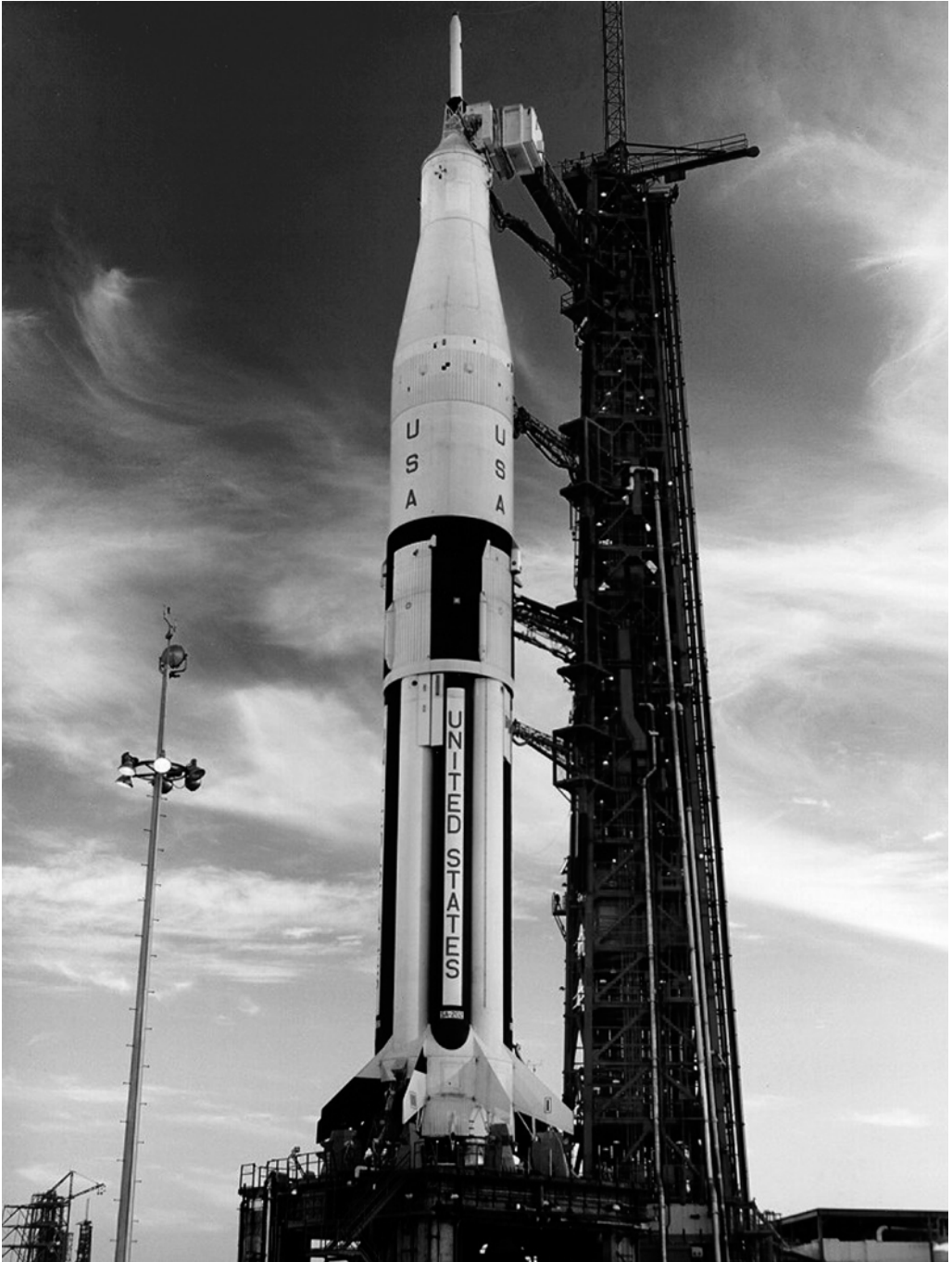
The Saturn IB is prepared for launch with the Block I spacecraft CSM-011.
