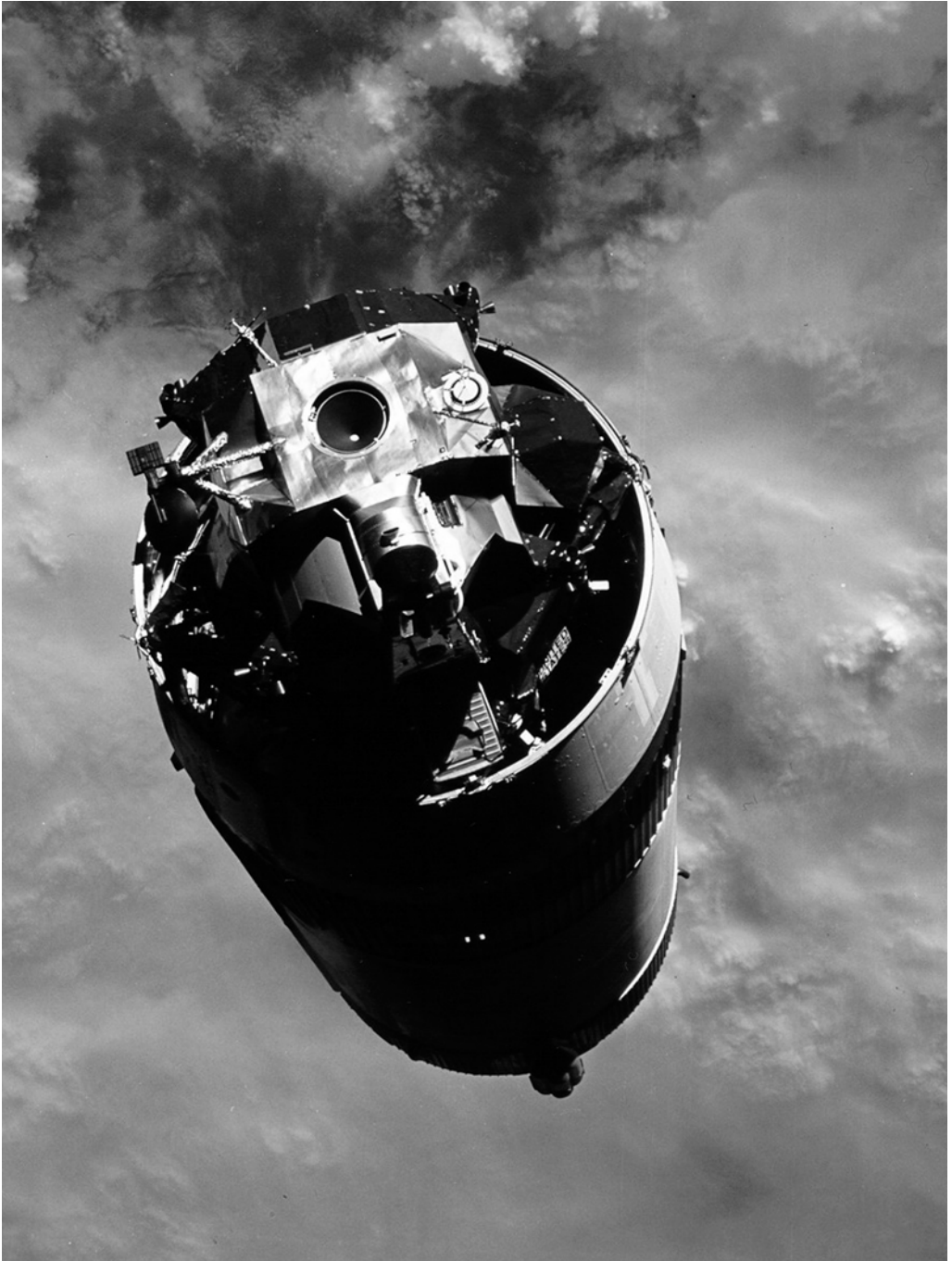
Apollo 9's spent S-IVB with its SLA panels jettisoned to expose LM-3.
