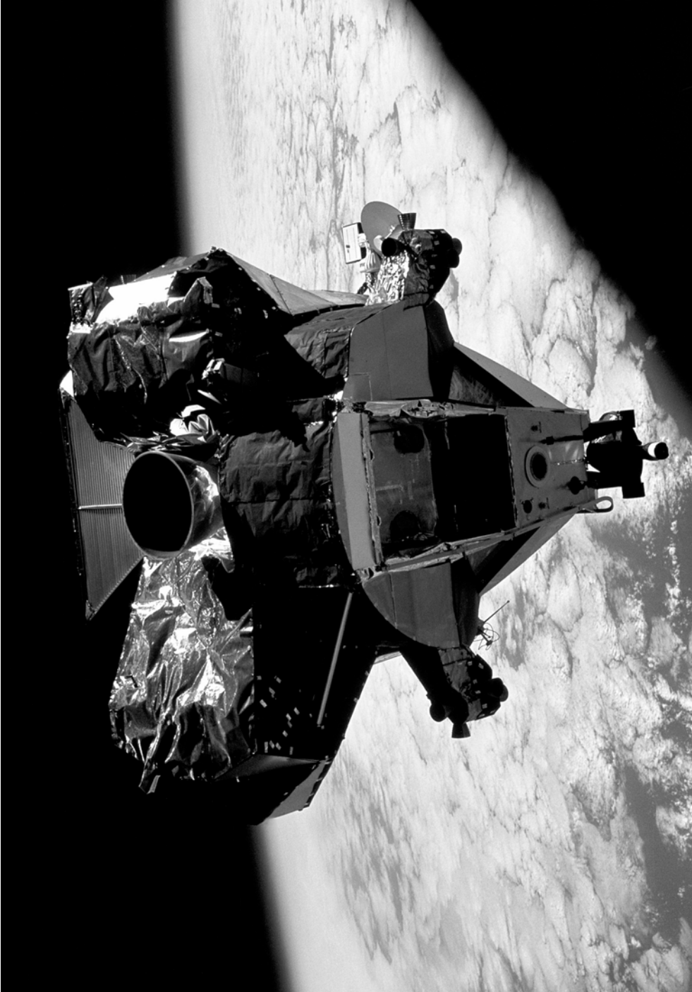
On returning from its independent mission, 'Spider' exposed its ascent engine to inspection.
