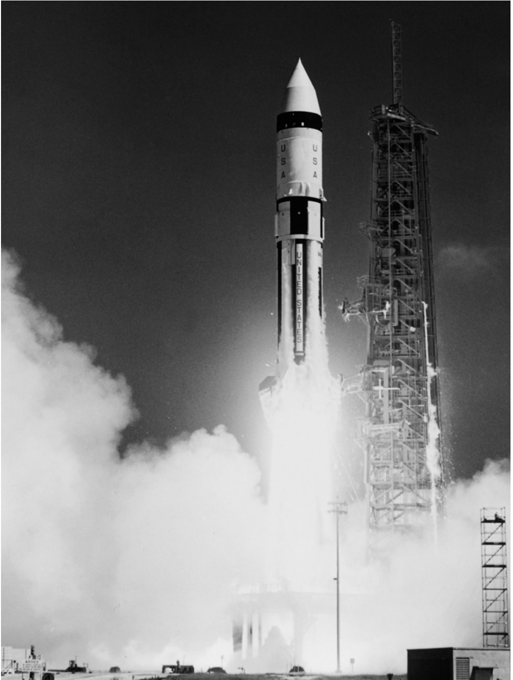
Lifting off without a spacecraft, AS-203 was to test the S-IVB stage in orbit.
