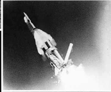
When the Little Joe II booster broke up during abort test A-003 on 19 May 1965, the launch escape system self-triggered to save the “boilerplate” spacecraft BP-22.
