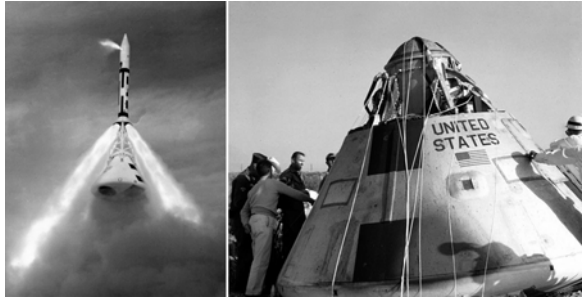
On 7 November 1963 the launch escape system lifts Apollo spacecraft BP-6 clear in its first 'pad abort' test (PA-1).
