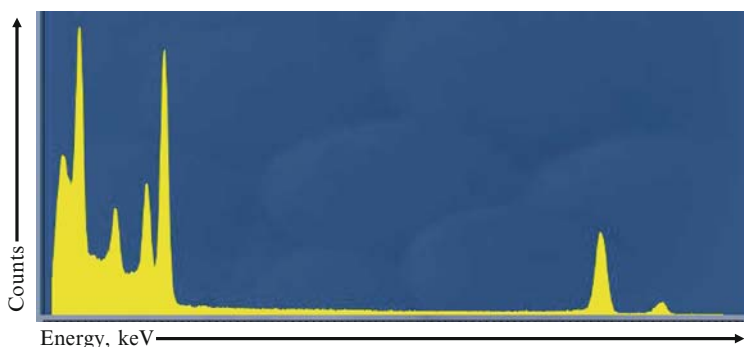
Fig. 4.16 Typical spectrum from energy dispersive spectrometry (EDS) analysis presenting Gaussian peaks at characteristic energies
