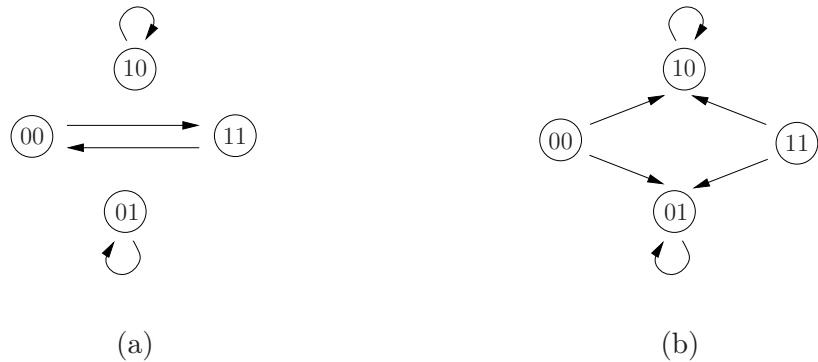
Figure 7.8 Transition graphs for the Boolean network corresponding to the cross-inhibition network (figure 7.7a). (a) Transition graph for synchronous transitions ( \rightarrow_s ). (b) Transition graph for asynchronous transitions ( \rightarrow_a ).
