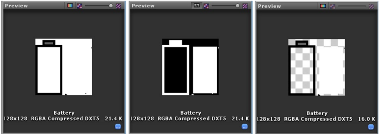
Figure 9-7. The “Texture” Texture Type (left), its alpha channel (center), and the “Sprite” Texture Type (right)
