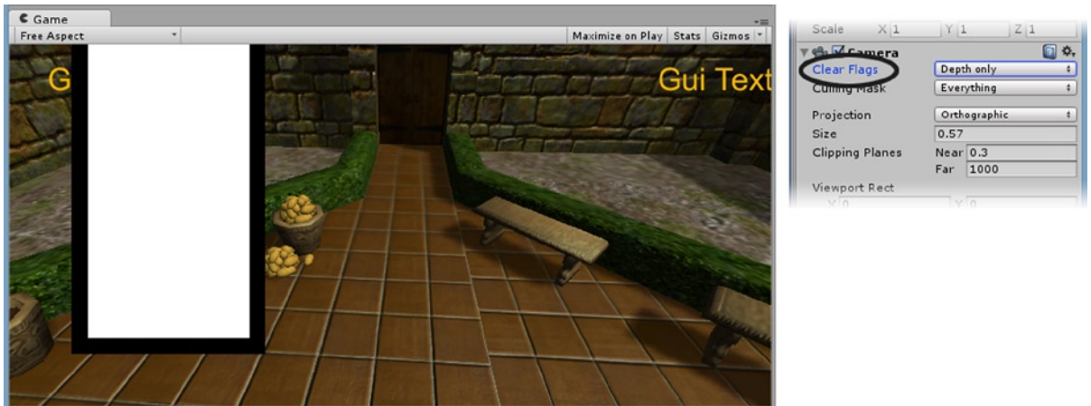
Figure 9-21. Depth only on the Camera GUI, allowing the Main Camera's view to show through
