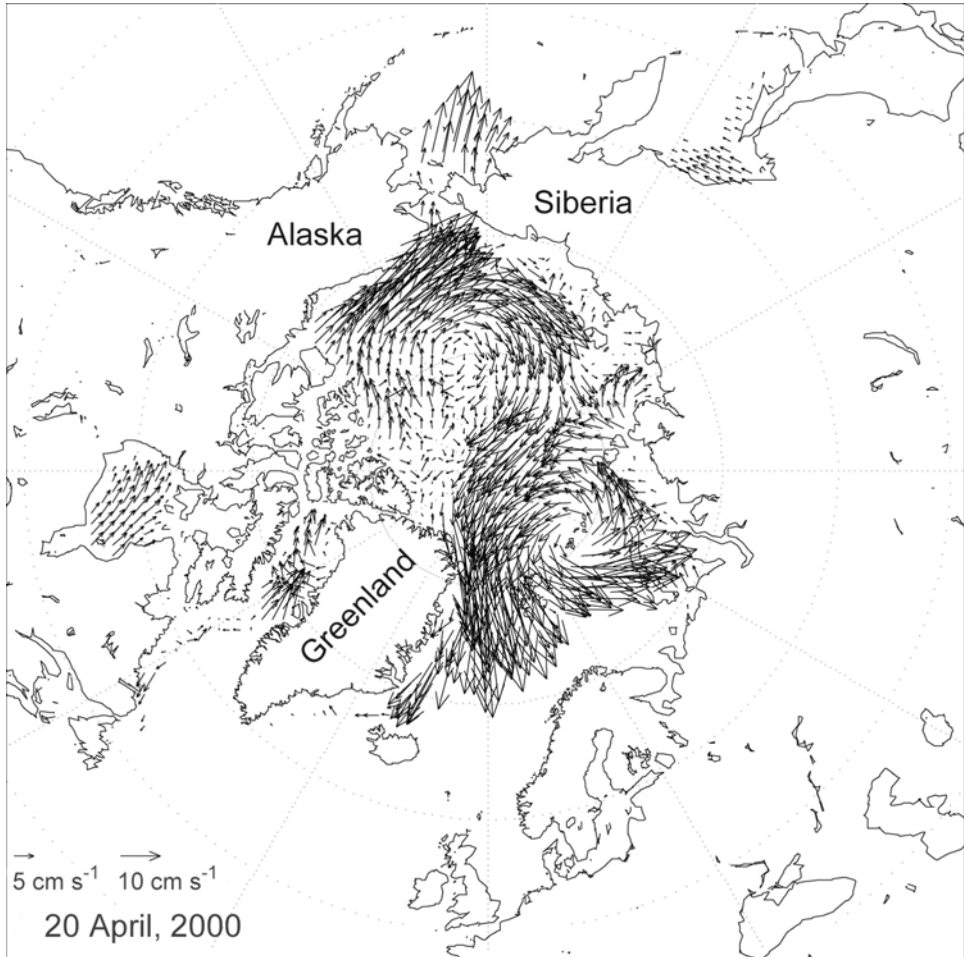
Figure 5.77. An example of a daily composite ice motion vector map from the NSIDC, for the Arctic for April 20, 2000. The map was created by optimal interpolation of daily gridded ice motion fields from the AVHRR, SSM/I, and IABP buoy data. In this case, every fourth vector is plotted.
