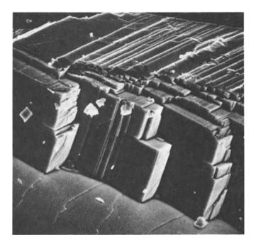
Figure 6.2. Photograph of a galena surface, after cleavage  $(160 \times)$ .
