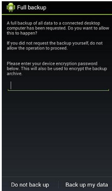
Figure 7-7. User interface option in an Android device when the ABD backup command is executed
