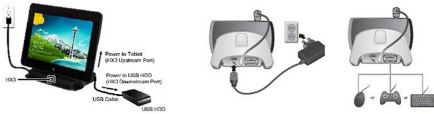
Figure A-4. A Cypress HX3 ACA dock (left) and Sony LiveDock docking device (right) (REF: User Guide)
