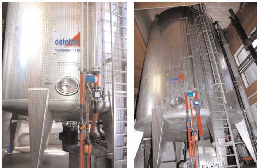
Figure 9.1 Example of a submerged vinegar fermenter with an annual production capacity of 18 million L of vinegar containing 10% acetic acid
