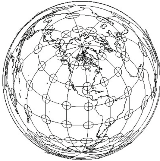
Fig. 6. Equal circles on the sphere are distorted in ellipses by projection from three to two dimensions. Circles are weak equivalent to the ellipses after the projection
