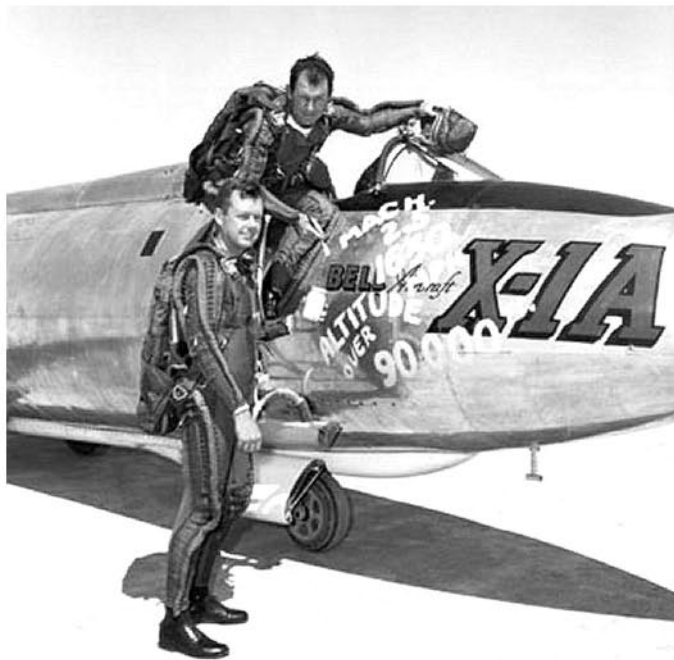
USAF test pilots Arthur 'Kit' Murray (standing) and Chuck Yeager wearing the DCC T-1 PPS pressure suit in 1954.
