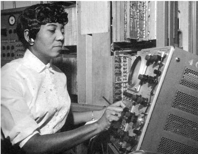
Dorothy B. John checks information put into a digital differential analyser. (Courtesy USAF.)
