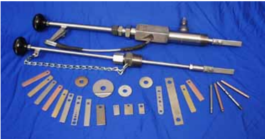
Examples of flat and cylindrical electric probes for corrosion control (doc Metal Samples)
