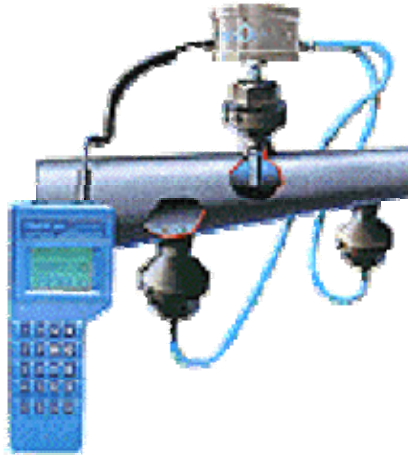
Electric measurement of corrosion (doc. Metal Samples)
