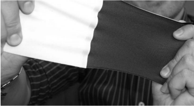
Fig. 3.12 Cotton joined to nylon using laser processing
