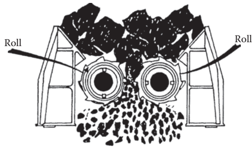
FIGURE 6.8 A double-roll crusher. (From Meyers, R.A., Ed., Coal Handbook , Marcel Dekker, New York, 1981, p. 188.)
