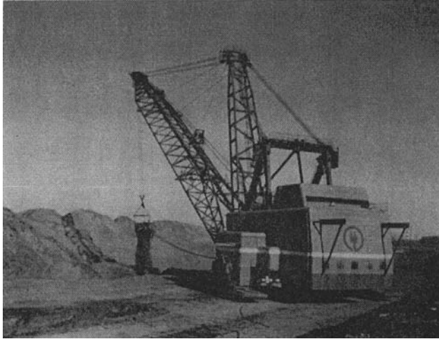
FIGURE 5.12 A dragline engaged in overburden removal. Weight: 7,000,000 lb, boom length: 425 ft, boom vertical height: 210 ft, and bucket capacity: 60 yd 3 .
