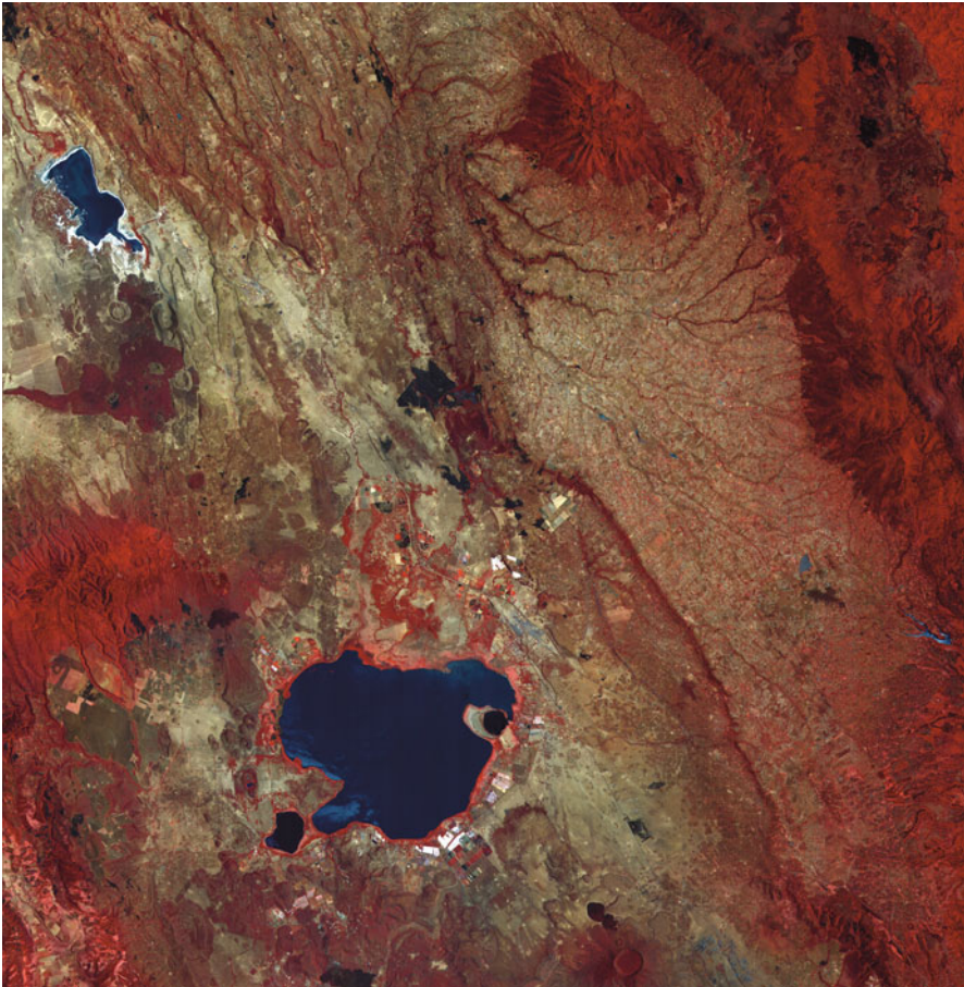
Fig. 8.4 RGB composite of a TERRA-ASTER image using the spectral infrared bands vnir_Band3n , 2 and 1. The result is displayed using imshow . Original image courtesy of NASA/GSFC/METI/ERSDAC/JAROS and U.S./Japan ASTER Science Team.
