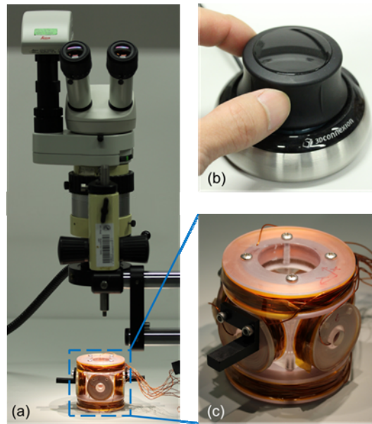
Fig. 8. Helmholtz coil setup to drive the micro-screw. (a) Tri-axis Helmholtz coil setup is used to drive and steer the micro-screw. Stereo-microscope (Leica MZ95 stereoscope with a Leica DFC 490 camera) is used to observe the movement. (b) 3-dimensional navigation of the micro-screw can be realized by turning the magnetic field with a joystick. (c) Enlarged picture of the tri-axial Helmholtz coil.
