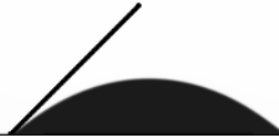
Figure 62. Multicomponent fluids interacting with a surface when G = 0.1 , G_{ads}^1 = -0.02 , and G_{ads}^2 = 0.0507 . The density of the first substance (with index 0) is show in gray scale. Line indicates 45^\circ contact angle. Simulation domain 1000 \times 200 lu^2 . Image represents 38,000 time steps from an initial condition of a 200 \times 50 lu^2 rectangle of the first substance (with density 1 and complementary density 0) surrounded by the second substance. \tau = 1 for both fluids.
