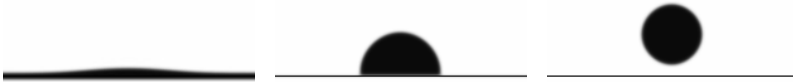
Figure 52. Simulation of 0, 90, and 180 degree contact angles based on the force balance rationale discussed in the text. For the cohesive interaction parameter G = -120 and the \psi function parameters \psi_0 = 4 and \rho_0 = 200 , G_{ads} = -327.79 , -187.16 , and -46.534 respectively.
