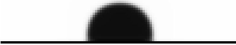
Figure 61. Multicomponent fluids interacting with a surface when G = 0.1 and G_{ads}^1 = G_{ads}^2 = -0.01 . The density of the first substance (with index 0) is shown in gray scale. Contact angle is 90^\circ . Simulation domain 100 \times 100 \text{ lu}^2 . Image represents 6000 time steps from an initial condition of a 20 \times 20 \text{ lu}^2 square of the first substance (with density 1 and complementary density 0) surrounded by the second substance. \tau = 1 for both fluids.
