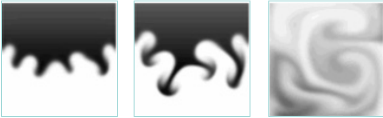
Figure 77. Solute induced buoyancy. A fluid containing solute is placed above a solute-free fluid in a gravitational field.
