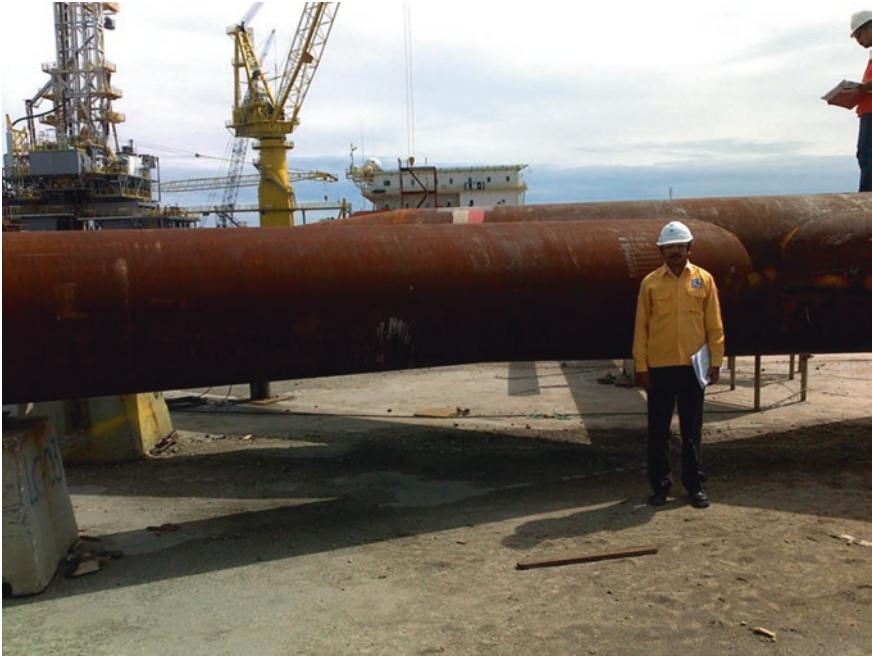
Fig. 7.1 Tubular component of a brace member assembly
