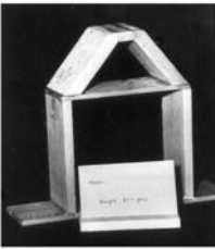
(c) Structure mass 87.7 gm failed at 522 N
