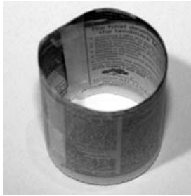
Figure 4.13(b) Cylindrical collar crushing specimen
