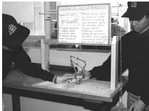
Figure 8.17 Conservation of angular momentum demonstration
