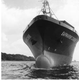
Figure 8.29 Bulbous bow on vessels in dry dock and at sea
