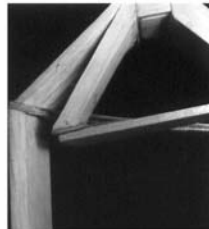
(c) Structure mass 87.7 gm failed at 522 N
