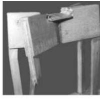
(a) Structure mass 84.8 gm; failed at 530 N
