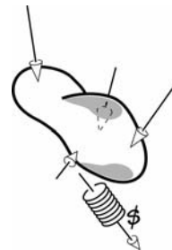
Figure A5 General system of forces acting on a body
