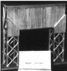
(e) Mass 28.5 gm, failed at 505 N
