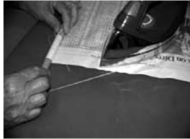
Figure 4.14 Paper column construction
