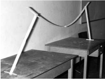
Figure 5.3 Simple suspension model
